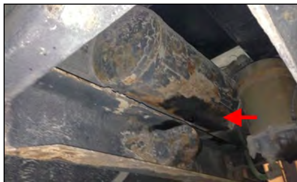
FIGURE 9: APPLICATION DE TECTYL 185GW BLACK
