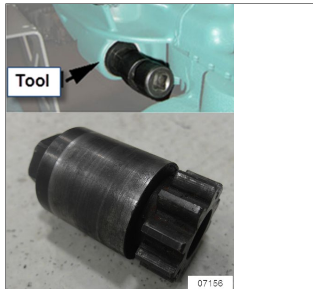
FIGURE 10: VOLVO ENGINE TURNING TOOL #88800014
