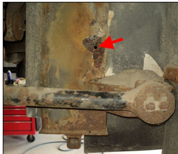
FIGURE 7: HOLE DRILLED IN STRUCTURAL MEMBER
