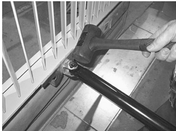
FIGURE 65: DOOR LATERAL ADJUSTMENT
