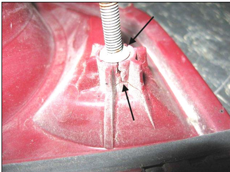
FIGURE 2: Cracks at the boss and ribs due to the use of engine degreaser
