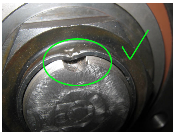
FIGURE 24: CORRECT - PREVENTS THE NUT FROM GETTING LOOSE
