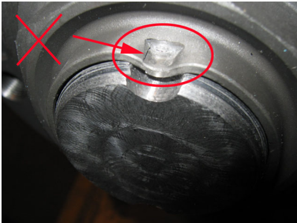
FIGURE 26: BROCKEN OR TORN LIP – REJECTED
