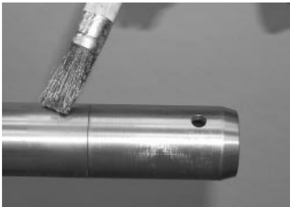
FIGURE 19: APPLY GLEITMO 805 GREASE
