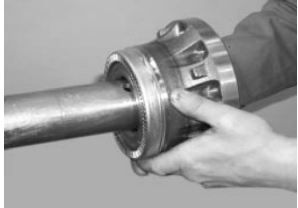
FIGURE 20: SLIP UNITIZED HUB BEARING OVER SPINDLE
