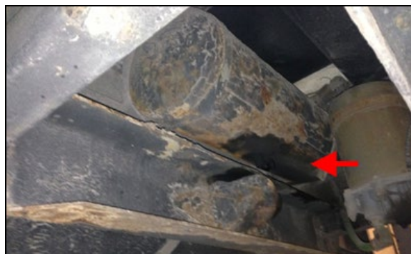
FIGURE 9: APPLICATION DE TECTYL 185GW BLACK
