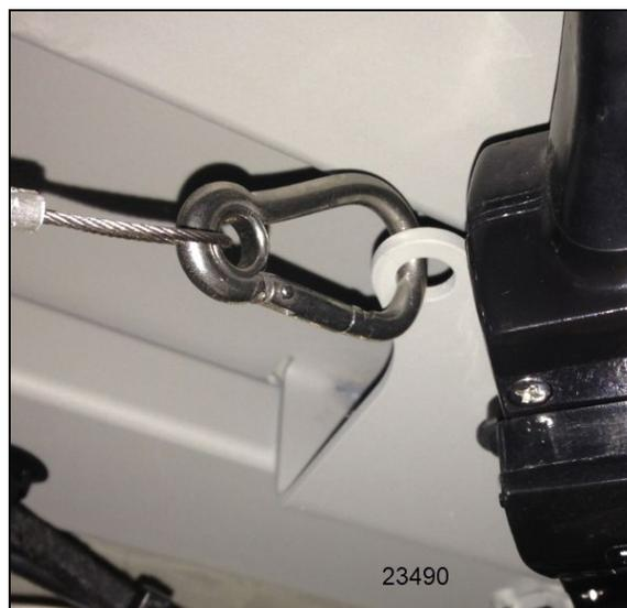
FIGURE 56: INSTALLATION DU CÂBLE DE SÛRETÉ
