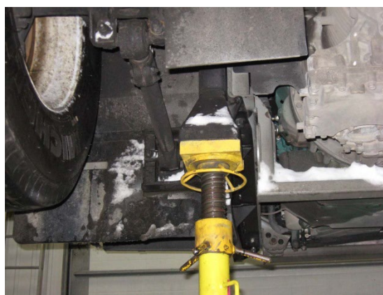
FIGURE 20 : JACK STAND AT CHASSIS HOISTING RECEPTACLE - AFT OF TAG AXLE, CURB SIDE
