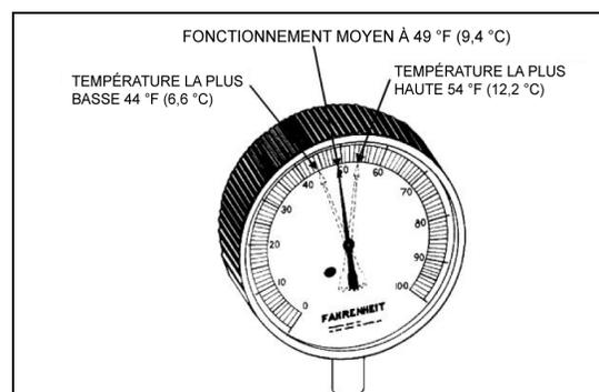
FIGURE 73: OSCILLATION DE TEMPÉRATURE HAUTE ET BASSE AU BULBE DISTANT
