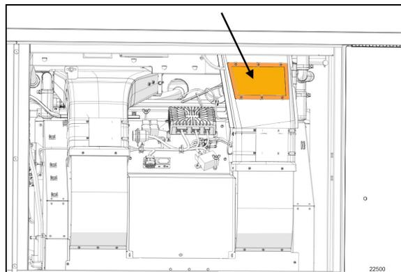
FIGURE 106: COUVERCLE D'ACCÈS DES MODULES DANS LE COMPARTIMENT ÉVAPORATEUR
