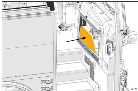
FIGURE 105: RETIRER LE COUVERCLE AVANT DU VENTILATEUR POUR ACCÉDER AUX MODULES
