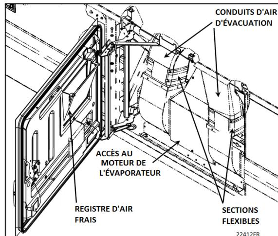
FIGURE 55: COMPARTIMENT DE L'ÉVAPORATEUR SÉRIE X3
