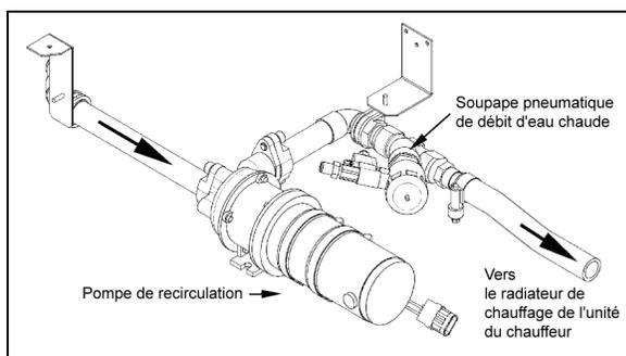
**FIGURE 78: INSTALLATION DE LA POMPE DE CIRCULATION D'EAU CHAUDE (PETIT SYSTÈME DE CVC)**
