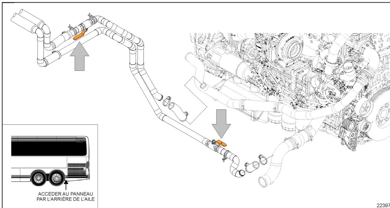
FIGURE 92 ROBINETS D'ARRÊT DE LA LIGNE DE CHAUFFAGE DE LA SÉRIE X3 (DISPOSITION DE TUYAUTERIE DE TRANSMISSION ALLISON ILLUSTRÉE)
