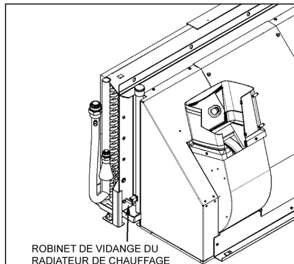
FIGURE 94: EMBLACEMENT DU ROBINET DE VIDANGE DU RADIATEUR DE CHAUFFAGE
