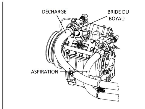
FIGURE 42: FLEXIBLE D'ASPIRATION ET DE REFOULEMENT
