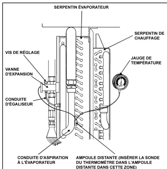
FIGURE 72: AJUSTEMENT DE LA SURCHAUFFE. INSTALLATION
