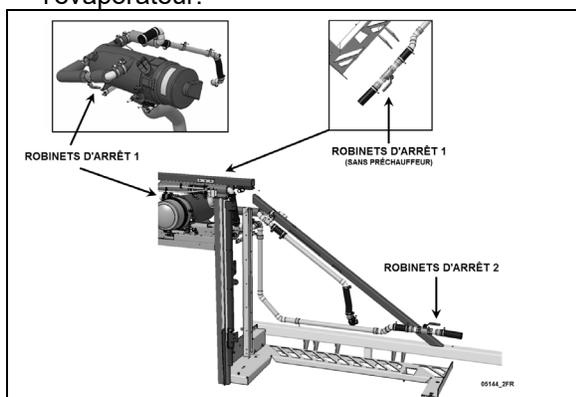
FIGURE 93: ROBINET D'ARRÊT DE LA CONDUITE DE CHAUFFAGE DE LA SÉRIE H3
