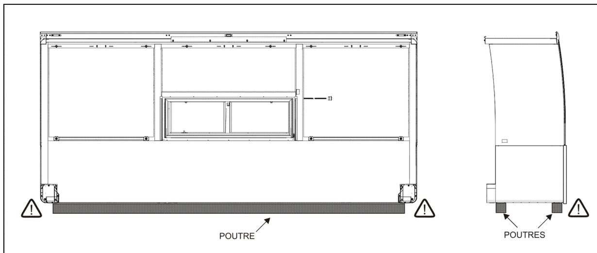
FIGURE 1: BEAM PLACEMENT
