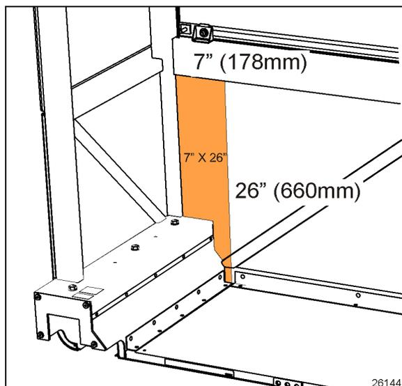
FIGURE 70: ZONE D'INTERDICTION DE PERÇAGE (AVANT ET ARRIÈRE)
