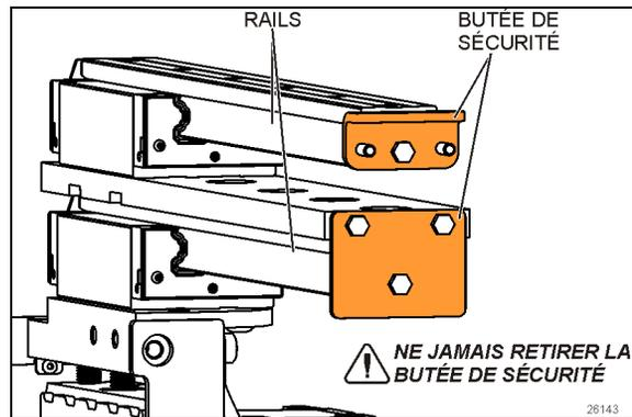
FIGURE 11: BUTÉES DE SÉCURITÉ SUR LES RAILS
