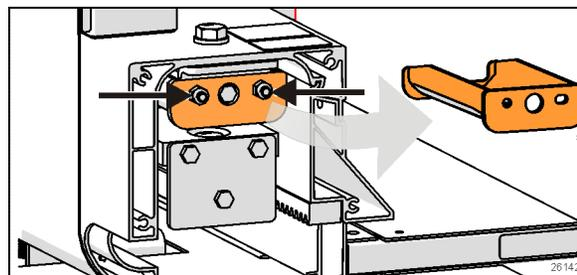
FIGURE 10: ENLÈVEMENT DE LA BUTÉE D'EXTENSION
