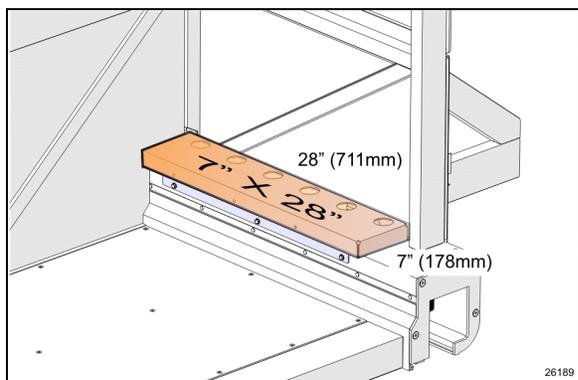
FIGURE 50: ZONE DE PERÇAGE INTERDIT, RALLONGE AVANT DROITE
