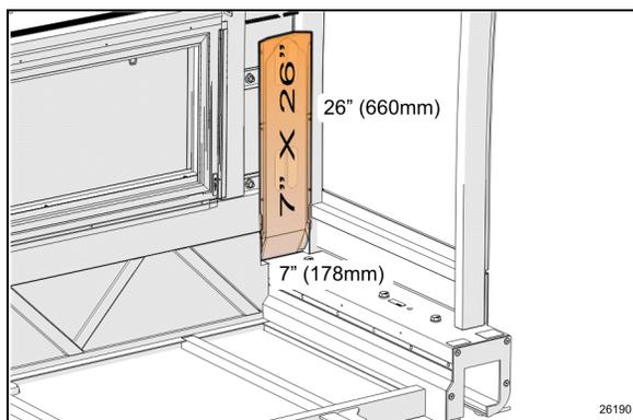
FIGURE 51: ZONE DE PERÇAGE INTERDIT, RALLONGE ARRIÈRE GAUCHE
