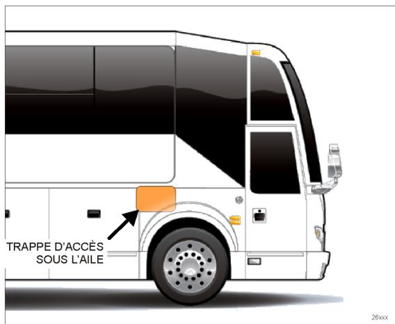
FIGURE 62: TRAPPE D'ACCÈS POUR LES VIS D'AJUSTEMENT POUR L'INCLINAISON ET MISE À NIVEAU
