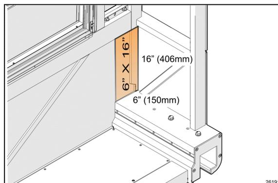
FIGURE 52: ZONE DE PERÇAGE INTERDIT, RALLONGE ARRIÈRE DROITE
