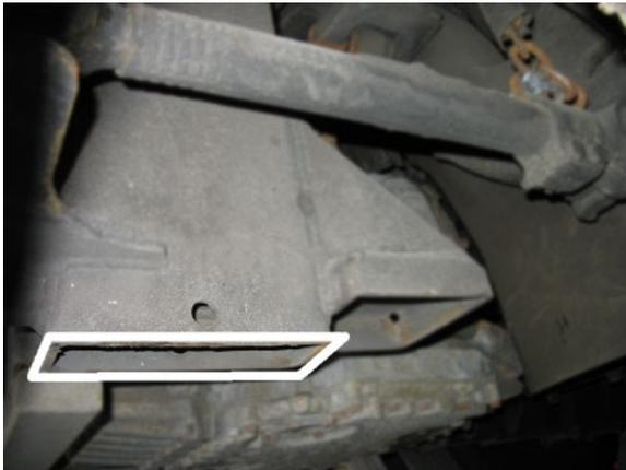
FIGURE 3: POINTS DE LEVAGE DU CHÂSSIS
