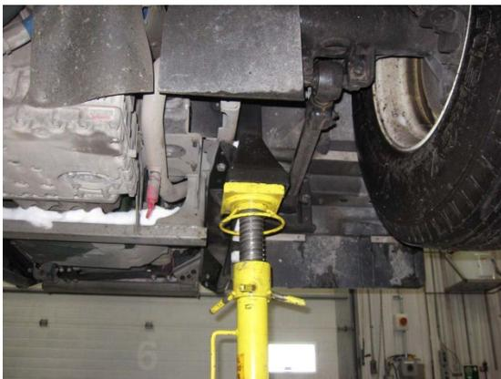
**FIGURE 19: CHANDELLE AU SUPPORT DE LEVAGE - À
