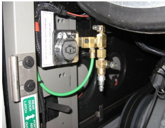
FIGURE 23: VALVE DE REMPLISSAGE DE SECOURS DANS LE COMPARTIMENT MOTEUR
