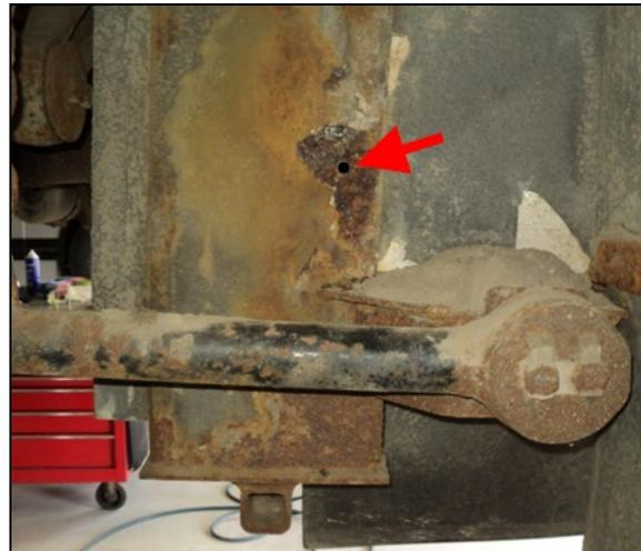
FIGURE 7: TROU PERCÉ DANS LE CHÂSSIS
