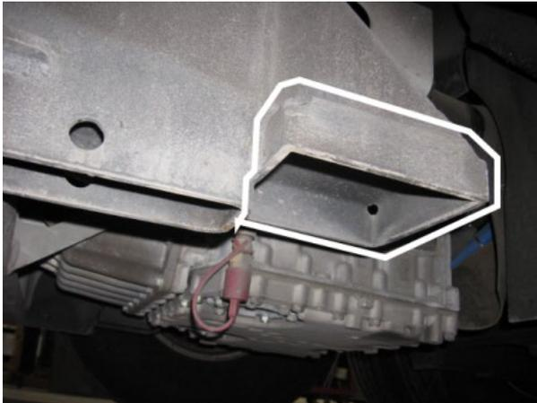
**FIGURE 15: SUPPORT DE LEVAGE AU CHÂSSIS
