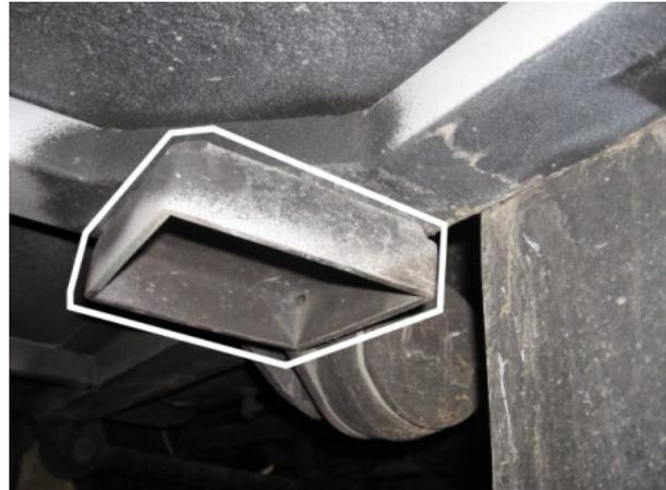
**FIGURE 16: SUPPORT DE LEVAGE AU CHÂSSIS
