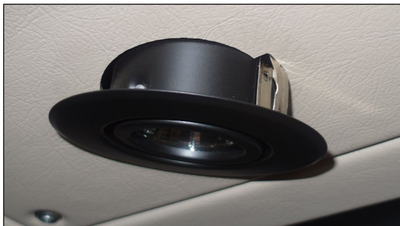
FIGURE 126: DRIVER'S AREA CEILING LIGHT
