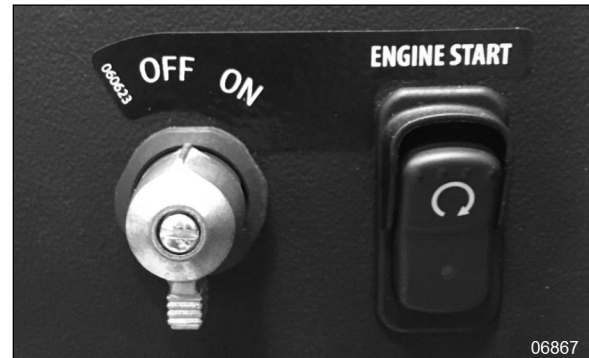
FIGURE 65: SWITCH ARRANGEMENT WITH STARTING MODULE
