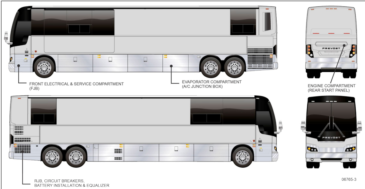
FIGURE 20: ELECTRICAL COMPARTMENTS (X3-45 VIP COMMERCIAL BUS SHELL)
