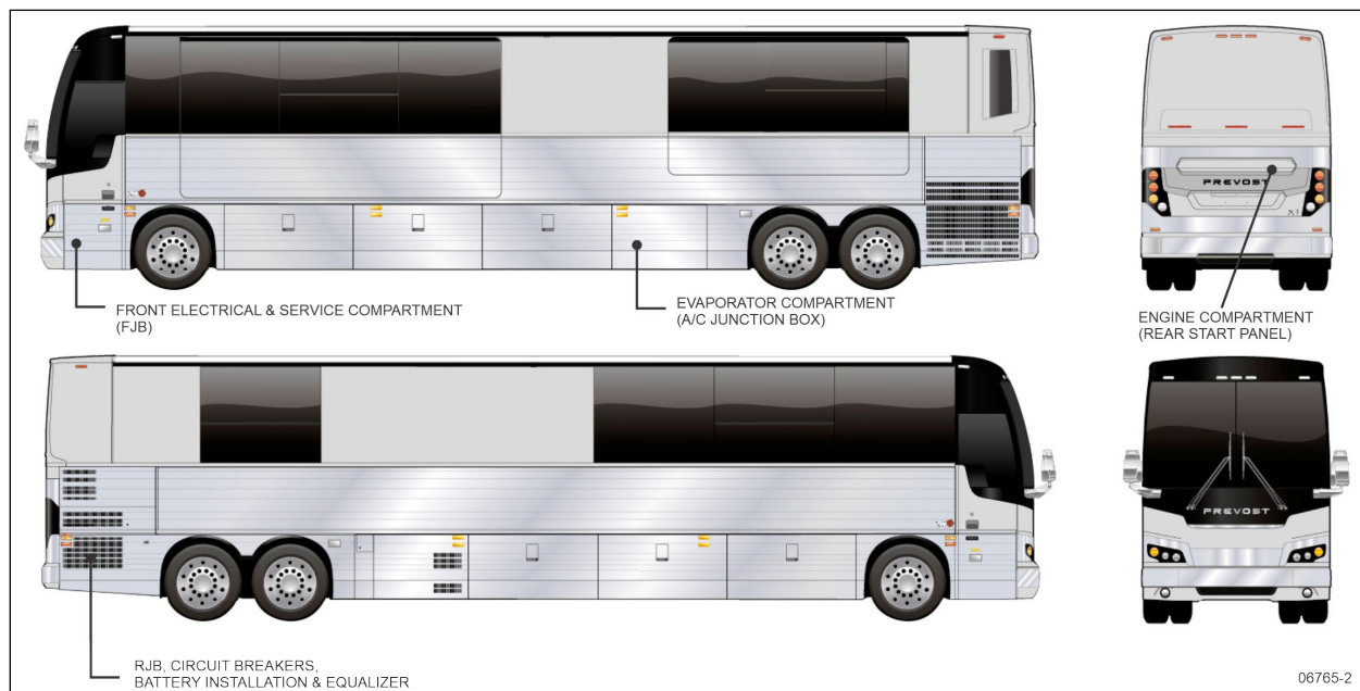
FIGURE 19: ELECTRICAL COMPARTMENTS (X3-45 VIP)
