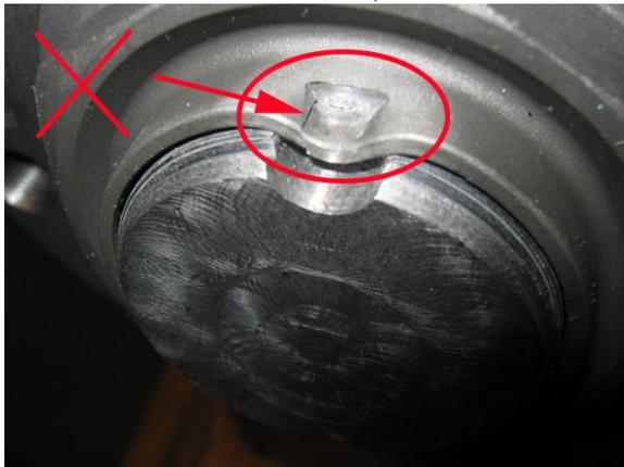
FIGURE 26: CREUX BRISÉ OU DÉCHIRÉE - REJETÉ
