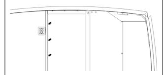
21. Place the foam tape 506001 along the metal extrusion as shown below.
