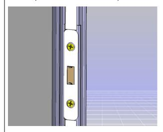
5. Cut the top of the metal extrusion as shown on the image below. It is very important to respect the 9/32" measure. The metal extrusion must lean against the track support in order to prevent any downward shifting of the track support which is screwed into fiberglass. This will prevent any malfunction caused by a misalignment of the sliding door locking mechanism and the strike plate, once properly adjusted.
