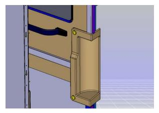
10.Remove the metal molding shown on the image below. This molding will not be reused. Keep the screws (4) for the installation of the replacement molding.
