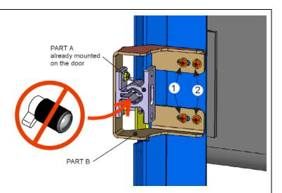
Discard the rubber cylinder, screw and plastic nut inserted inside the part shown on the image. They are not required.
