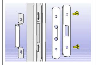
15. Dismount the door handle mechanism. Keep the internal mechanism for reuse. The 1/8" thick shim on the passenger's side will not be reuse. Two 1/16" thick shims 409286, one on each side, will be used instead. Install parts 409315 & 409316 as shown below. **Do not** tighten screws too much in order to permit free movement of the latching mechanism.
