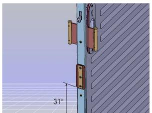
18. Cut the included Velcro 506756 in two pieces of 1"x1½". In order to absorb vibrations and noise, place the pieces on the door guiding blocks as shown on the image.
