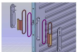
16. Remove the existing mechanism that holds the door closed when unlocked. Using the existing hardware and holes, install assembly 409295. The part of assembly 409295 shown on the image below must be installed on the door.
