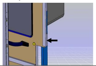
11. Using a jigsaw cut the particle board out as shown on image 10a & 10b. Prior to do so, apply masking tape on the surrounding surfaces to prevent scratches from the jigsaw base.
