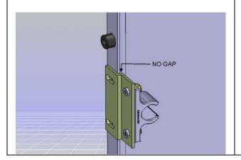
17. Install the rubber **vibration damper** 409309 with plate 409308 and 3 screws 500435. Install the vibration damper, properly centered, at 31 inches from the bottom of the door.
