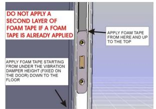
22. Proceed to the adjustment of the strike plate height. The lower edge of the rectangular opening must be at the level of the latch as shown. To do so, loosen the screws and move the strike plate up or down as required. Once properly adjusted, tighten the screws.
