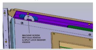
20. Install the left wall metal extrusion. In order to assure that the metal extrusion is properly positioned before screwing it, close and maintain the door firmly against it. This will help in finding out the proper positioning of the extrusion.
