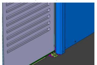
26. Reinstall the panel on the right side of the sliding door and all the remaining trims.
