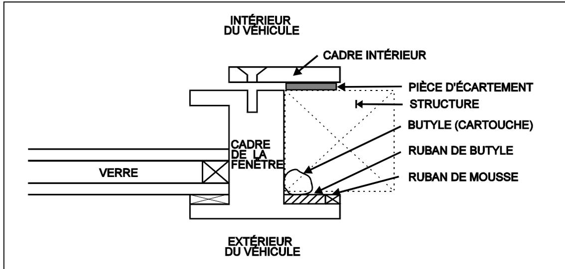
FIGURE 1: COUPE DE LA NOUVELLE FENÊTRE
