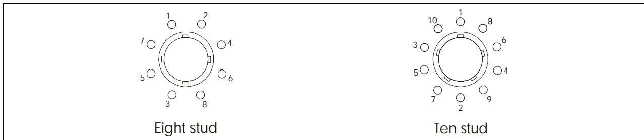
FIGURE 6: TIGHTENING SEQUENCE
