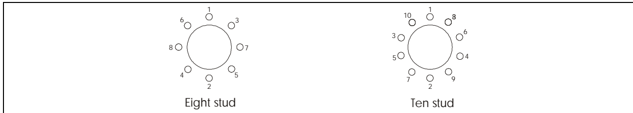
FIGURE 3: TIGHTENING SEQUENCE
