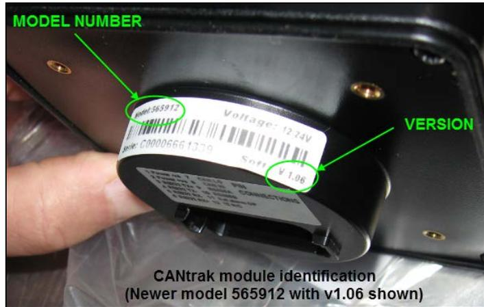
Fig.5 Model number & version (New model 565912 v1.06 shown)
