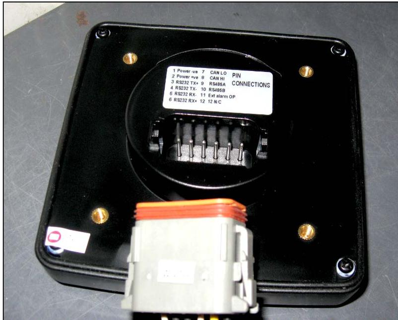
Fig.9 CANtrak module connection.
