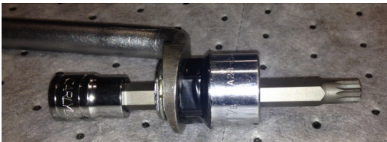
OFFSET 7/8 WRENCH FITTED WITH 7/8 SOCKET AND 10mm 12-POINTS SPLINE DRIVE
