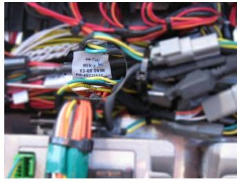
2. Disconnect electrical plug at the extinguisher to prevent any false triggering of the system.
