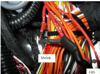
8. Splice a new white wire on the remaining end of wire 341.
