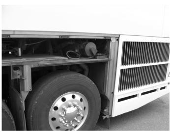
2. Inspect the clearance between the Preheater exhaust tube and the tag axle tire.
