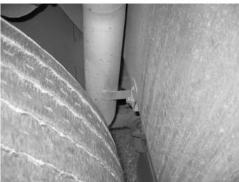
3. This is the correct position. Distance between tube and tire should be approximately 2 in.
