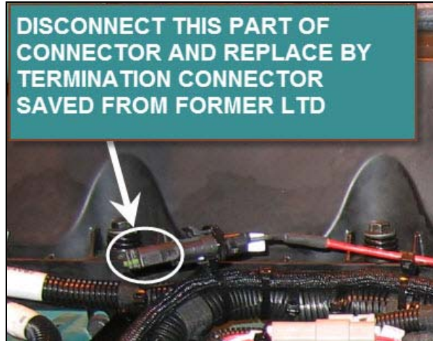
STEP 3 H: TERMINATION CONNECTOR
