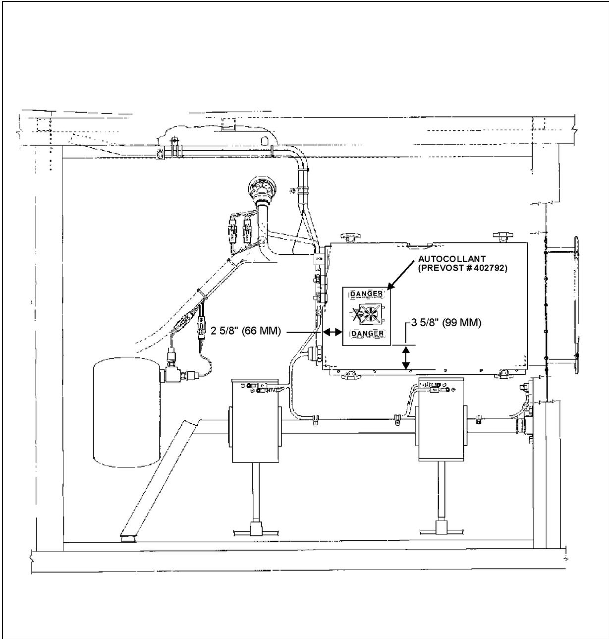
FIGURE 1: COMPARTIMENT DU CONDENSEUR
