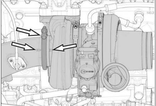
NOTE: WHEN POSITIONING THE DIFFUSER PIPE, ALIGN THE MATCH MARKS ON THE DIFFUSER AND ENGINE TURBOCHARGER, IF EQUIPPED
