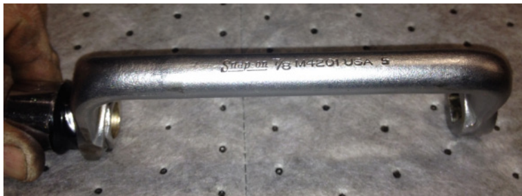
OFFSET 7/8 WRENCH (CYLINDER HEAD WRENCH), SNAP-ON PART NUMBER M4201
