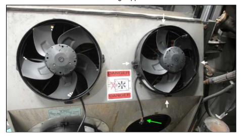
24. Position the adaptor ring over the lower (exterior) fan opening & hold the ring in place using two C-clamp pliers, make sure the ring is centered over the opening and that there's enough material around the ring rivet holes.
