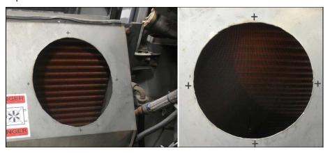
21. Center drill the four fan mounting holes & drill the four holes to their final diameter using a short 5/16" drill bit (deburr both sides of the drilled holes).
