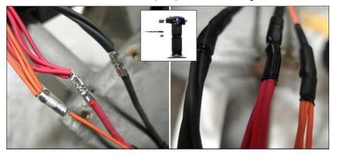
14. Connect the four fans to the new harness connectors (fans can be connected to any connector, connectors are interchangeable). Add cable ties (504637) to the harness as required to securely maintain it to the door structure.
