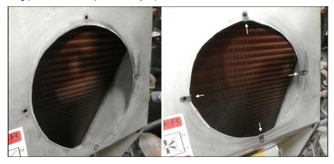
23. Position a fan over the opening, making sure the fan wiring harness is pointing toward the center of the shroud. Secure the fan to the shroud using supplied bolts and nuts.
