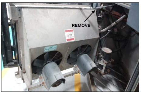
2. Remove the retaining strap bracket on the fan shroud (drill rivets).
