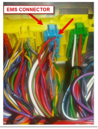
11) Extend BMUX/1, BMUX/2, BMUX\_1/3 using splice #956956 and corresponding color coded wire. IMPORTANT: Read the note below.
