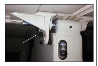
9. Reinstall the ball stud. Discard the washer on the nut side - Install both washers on the ball side.
