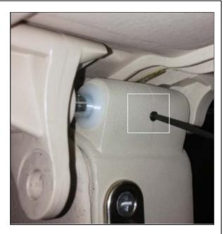
5. From inside the adjacent compartment, slowly slide the pivot rod out of the door support using locking pliers (do not mar the rod).
