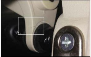
1. Open the door and disconnect the gas shock from the door support (use a small screwdriver to lift the retaining clip holding the shock head to the ball stud).
