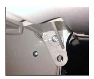
6. Insert the exterior (larger) reinforcing plate and slide back the pivot rod in place (center the rod 50% on each side).
