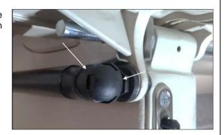
11. Push the door toward the interior to make sure that there is no interference between the ball stud nut and the parcel rack panel.
