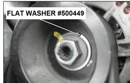
2. Make sure that the alternator pulleys do not slip. Make sure that the nuts are tight. **Correct if needed.**
