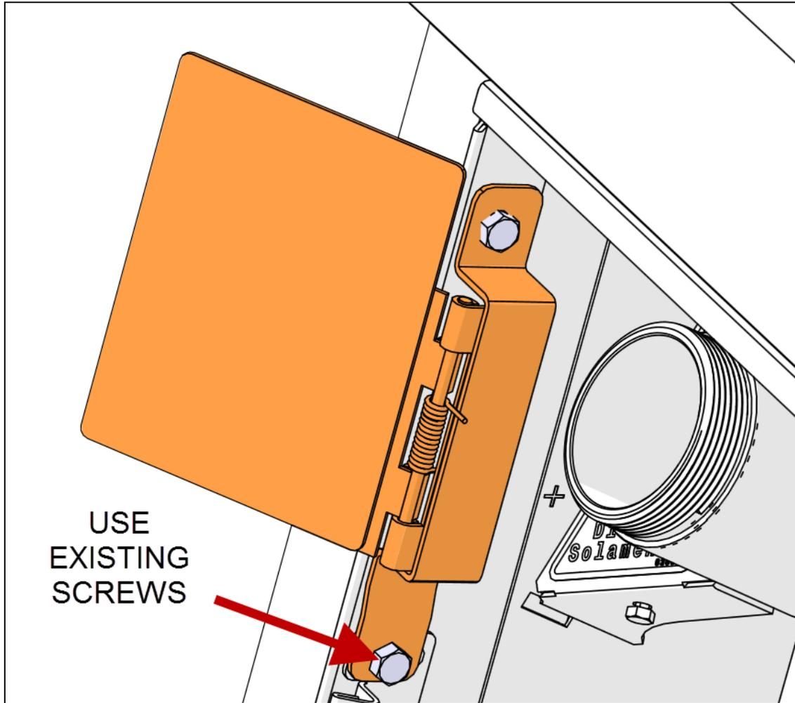
FIGURE 2 : X3 MODELS WITH LOCK MODELS FLAP INSTALLATION
