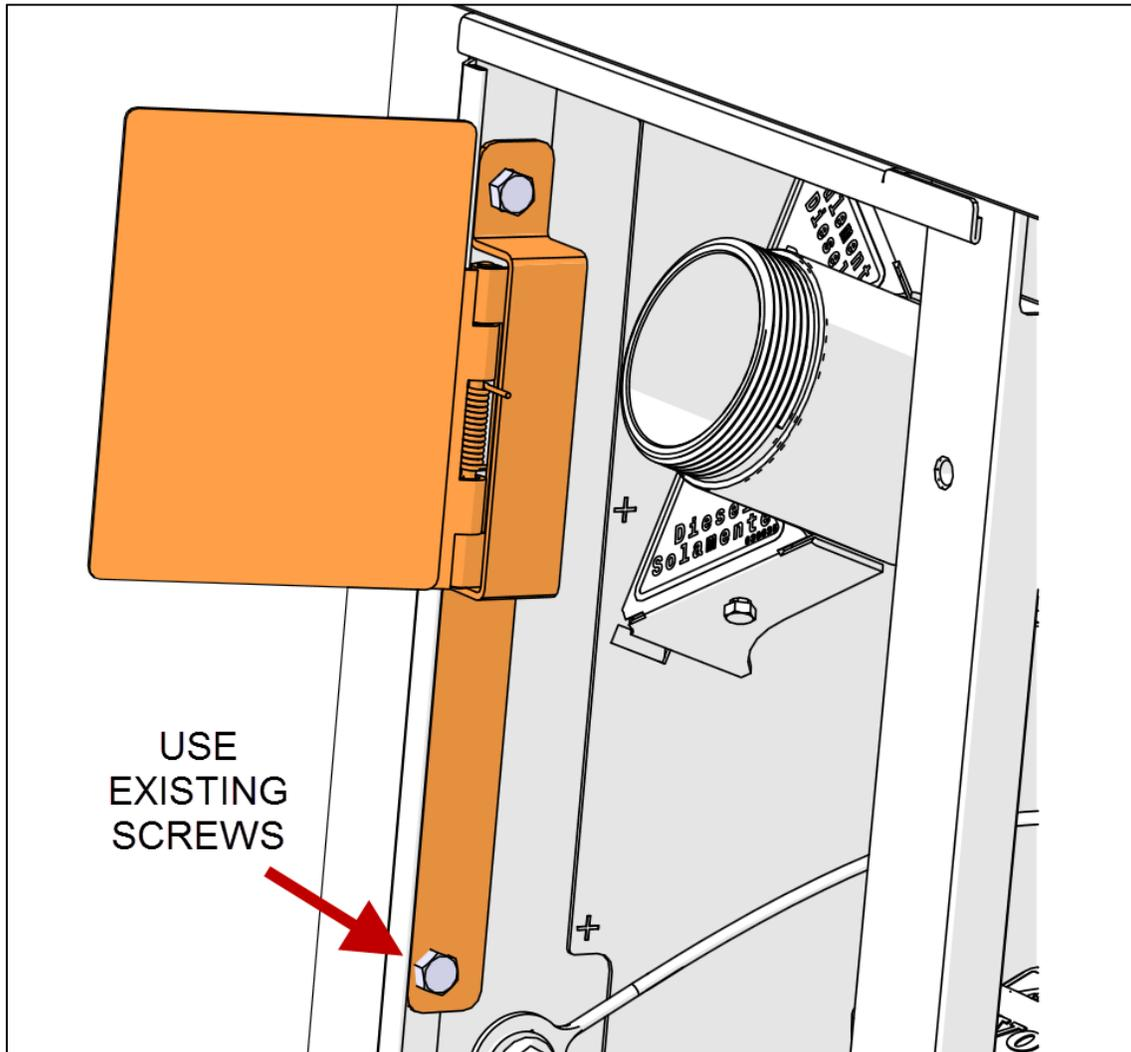
**FIGURE 3 : X3 MODELS WITHOUT LOCK FLAP INSTALLATION**
