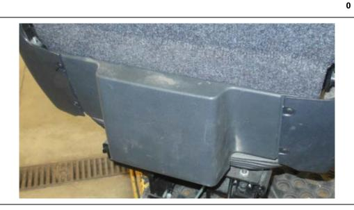
6. Connect the buckle harness to the vehicle (vehicles with connector under the seat).
