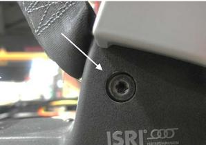
Make sure that the belt is centered in the top part of the sliding rail and that there is no belt to rail contact at the lower part of the rail. Adjust the angle of the seat belt mechanism as required.
