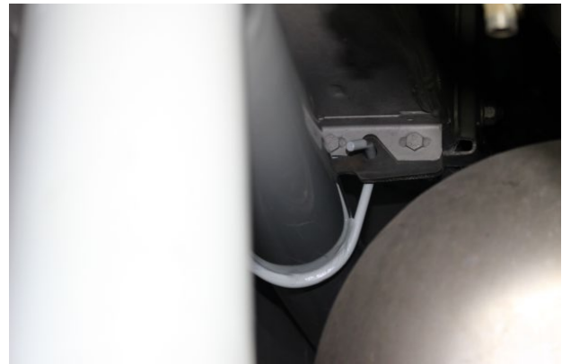
FIGURE 101: ENGINE INTAKE PIPE SUPPORT
