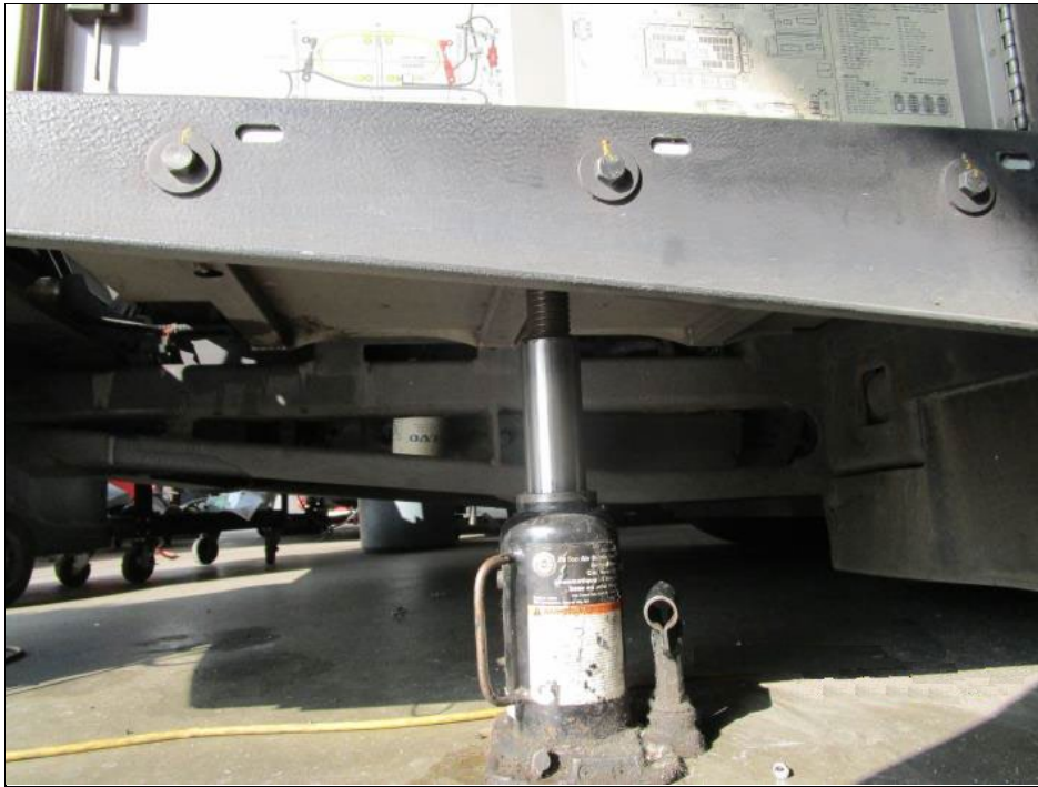
FIGURE 12: SUPPORTED BATTERY TRAY
