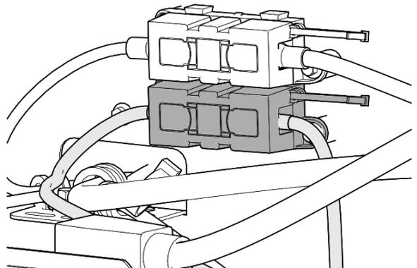
7. Make sure that the bottom battery charger fuse is rated 40A.
