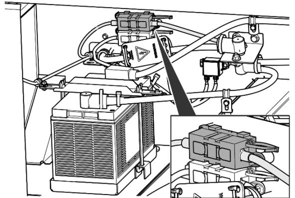
6. Remove the cap covering the lower battery charger fuse (press clips and pull off).
