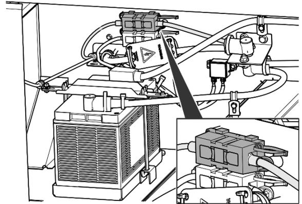
3. Make sure that the top battery charger fuse is rated 80A.
