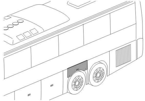
2. Remove the cap covering the top battery charger fuse (press clips and pull off).
