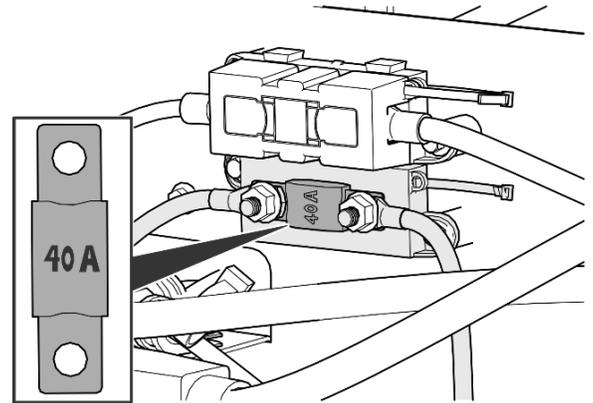
8. If the bottom fuse is not a 40A fuse, remove it and replace it with part # **60111397** (40A fuse).
