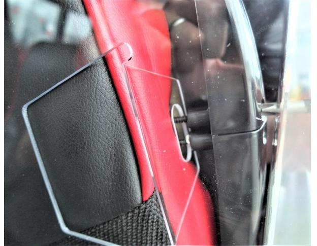
3. Reinstall the safety belt guide making sure that the two center screw bosses are inserted in the partition angled tab slot. Partially screw each 4 screws and tighten alternately until the guide is firmly secured. This will also hold the partition in place for the next steps.
