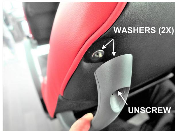
3. Remove the 4 screw that hold the safety belt guide on the opposite side of the seat.
