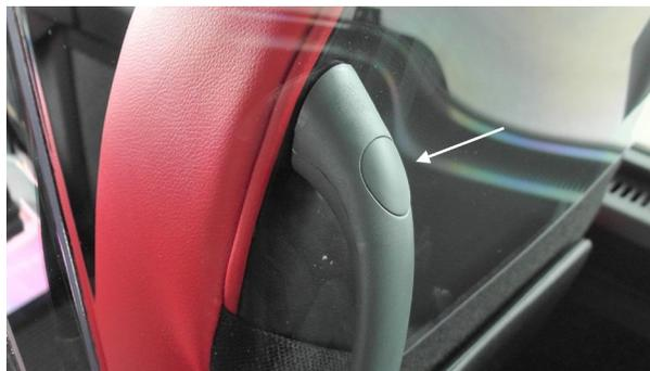
9. Left and right aisle partition: Install decal #7771102 centered on the lower part of the partition (installation with handles shown).
