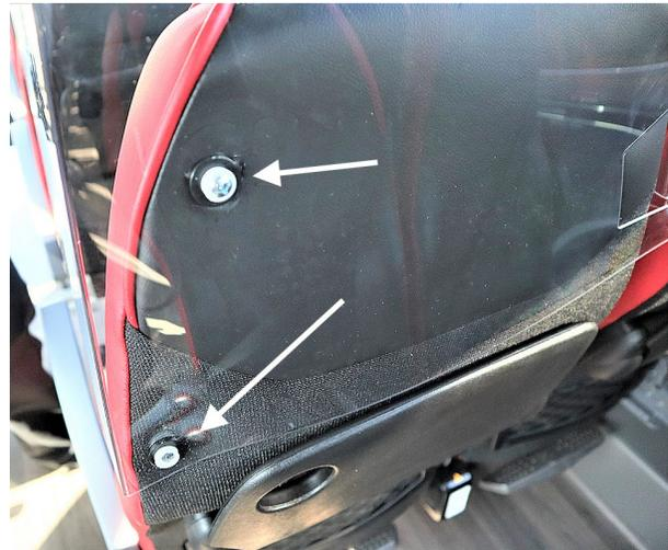
6. Clip the **#504400** plastic caps over the screw heads to finish the installation.
