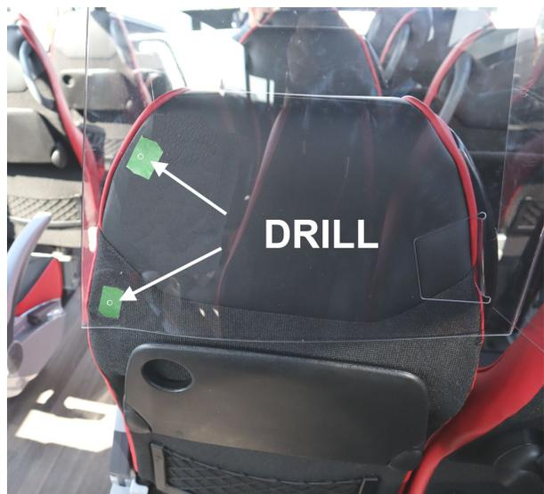
5. **FOR INSTALLATION USING SCREWS:**
