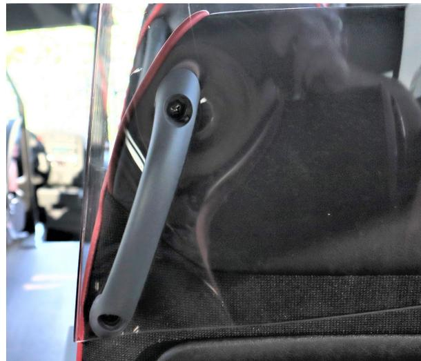
8. Install the handle screw caps to finish the handle installation.
