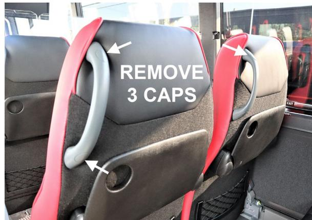
2. Unscrew the handle. If present, do not lose the 2 small washers that may be stacked between the seat body at the top handle mounting point.
