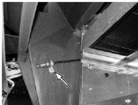
**40.** Remove the wedge was placed between defroster unit and at the bottom of its installation compartment for secure the defroster unit during air distribution box installation.
