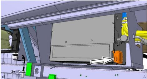
**52.** Open flux valve for driver area heating circuit.
