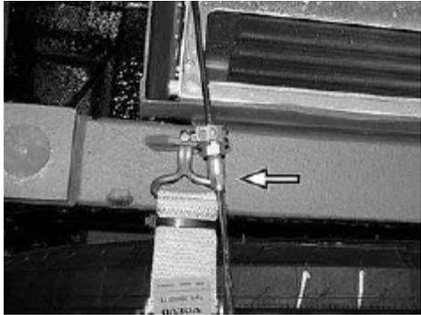
**49.** Check the coolant fluid level in the expansion tank.
