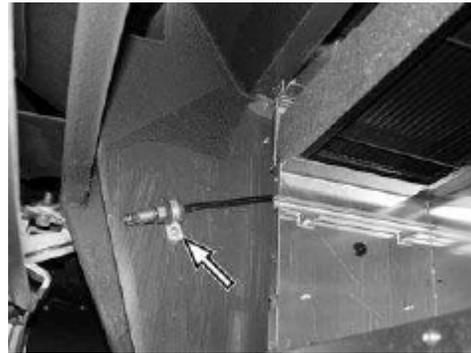
19. Drain coolant from defroster heater coil.
