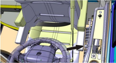
**53.** Perform A/C system refrigerant filling. See service operation: 87001-3 Refrigerant air conditioning system, fill; published in IMPACT, as a reference.
