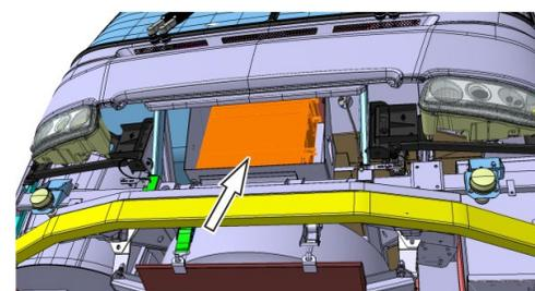
27. Install reinforcement L-profile **P/N: 23811261**. Welded at center and under front plate frame according separately assembly drawing document: **22314124 Frame front section DOT**, see annex on this service document as a reference.
