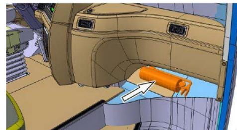
**67.** Install dashboard upper cover by screw its 8 fixing screws placed around at the cover contour.
