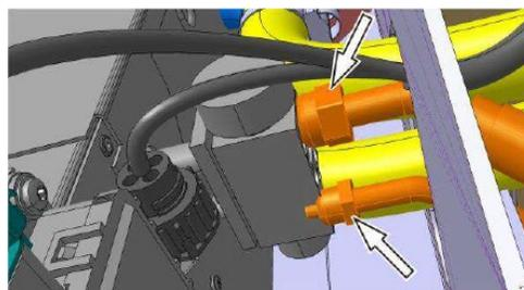
**42.** Install defroster expansion valve lower connection lock plate.
