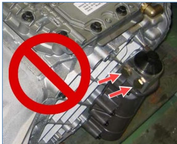
Figure 5: DO NOT BLOCK THE CONNECTION PORTS AT THE TOP OF THE OIL FILTER HOUSING
