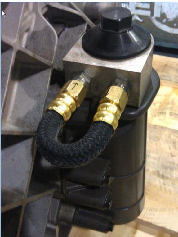
FIGURE 4: VOLVO 9700 – OIL CIRCULATION LOOP
