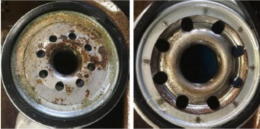
**Figure 4: CRYSTAL BUILDUP AND CORROSION/RUST PRESENT ON PRIMARY FILTER. CORROSION/RUST ON SECONDARY FILTER**
