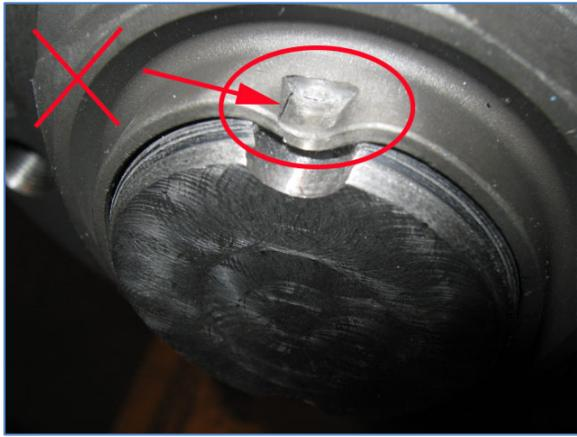
**Figure 32: BROCKEN OR TORN LIP – REJECTED**
