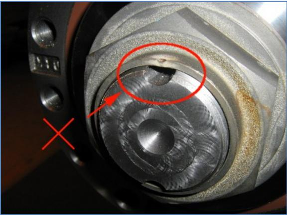
**Figure 33: LIP INADEQUATELY PRESSED IN – REJECTED**
