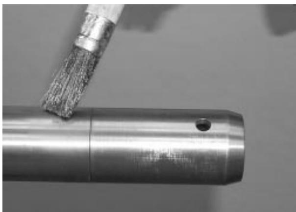
**Figure 25: APPLY GLEITMO 805 GREASE**
