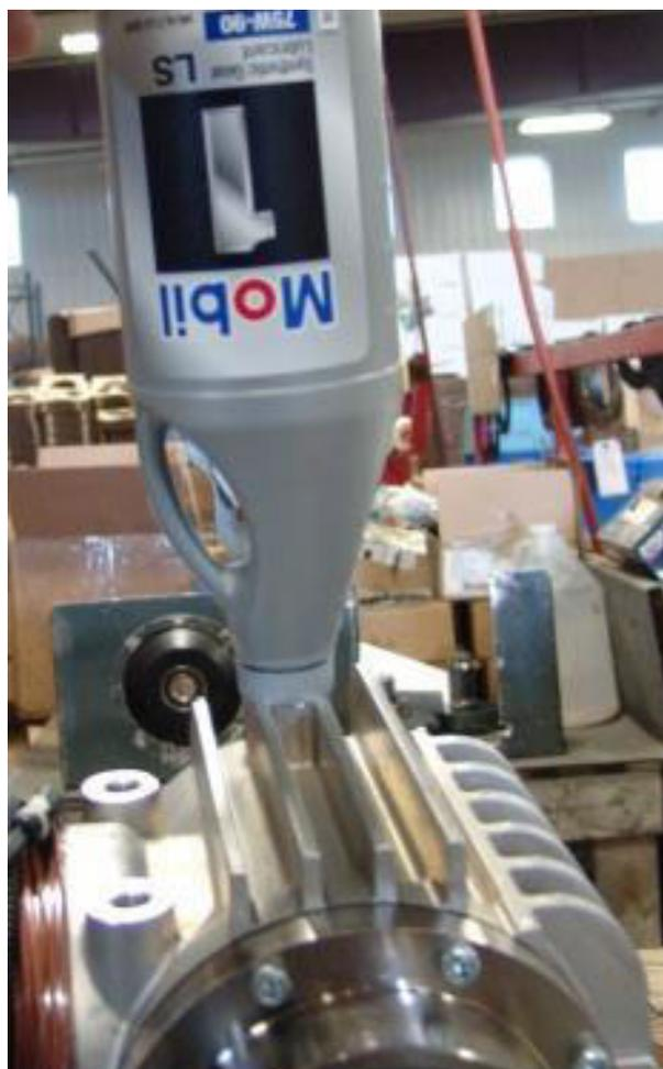
5. Reinstall breather/dipstick and check the oil level. If the oil is above the line on the dipstick reinstall, the oil change is completed.
