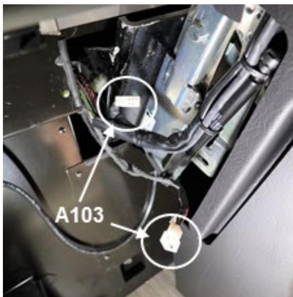
18. Using extractor tool **681485**, remove the ground wire **00A** located at PIN 4 of the A103 connector.
