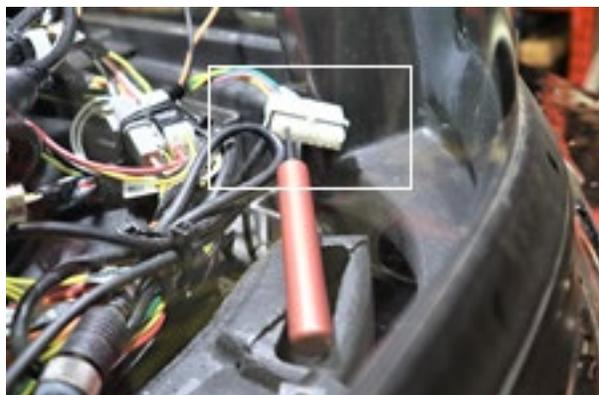
8. Cut the terminal from the end of the extracted wire and add a length of supplied shrink tubing to protect the end.
