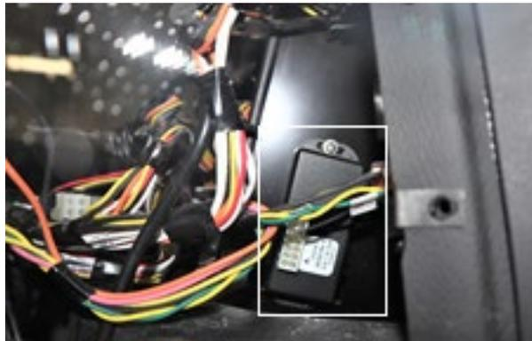
7. Using extractor tool **681485**, remove the terminals located at PIN 2 (A55RJ1.18 wire) from the A139 module connector.
