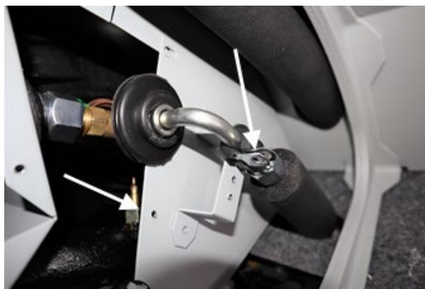
6. Disconnect the drain pipe at the back of the AC unit.
