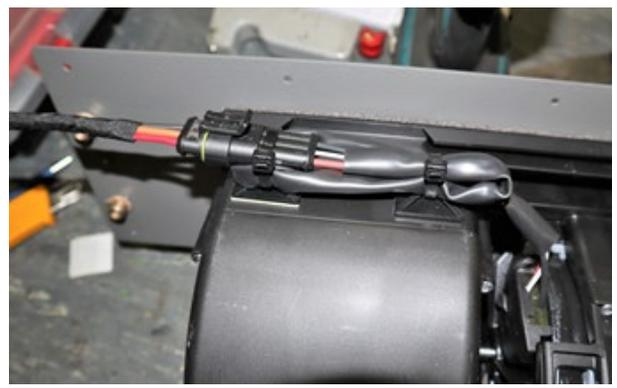
6. Secure the new blower assembly to the AC unit.
