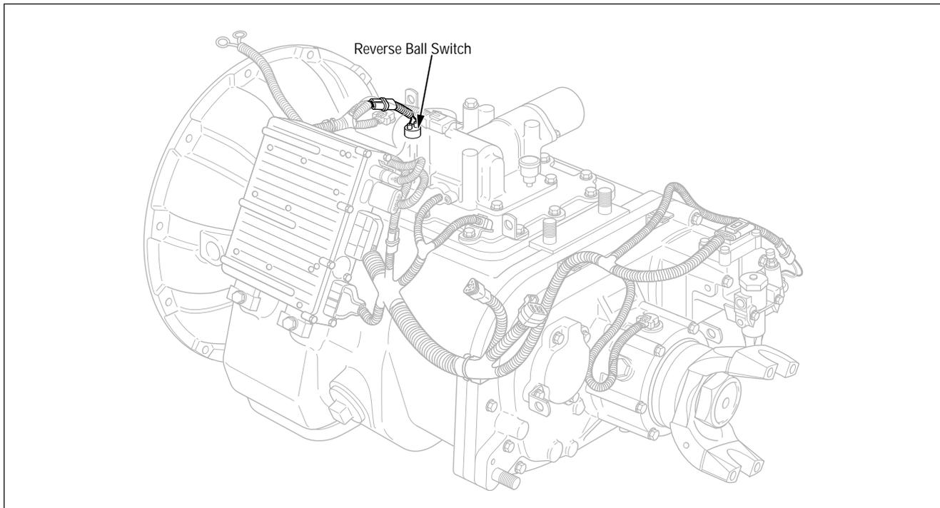
Figure 1. Reverse Ball Switch Location
