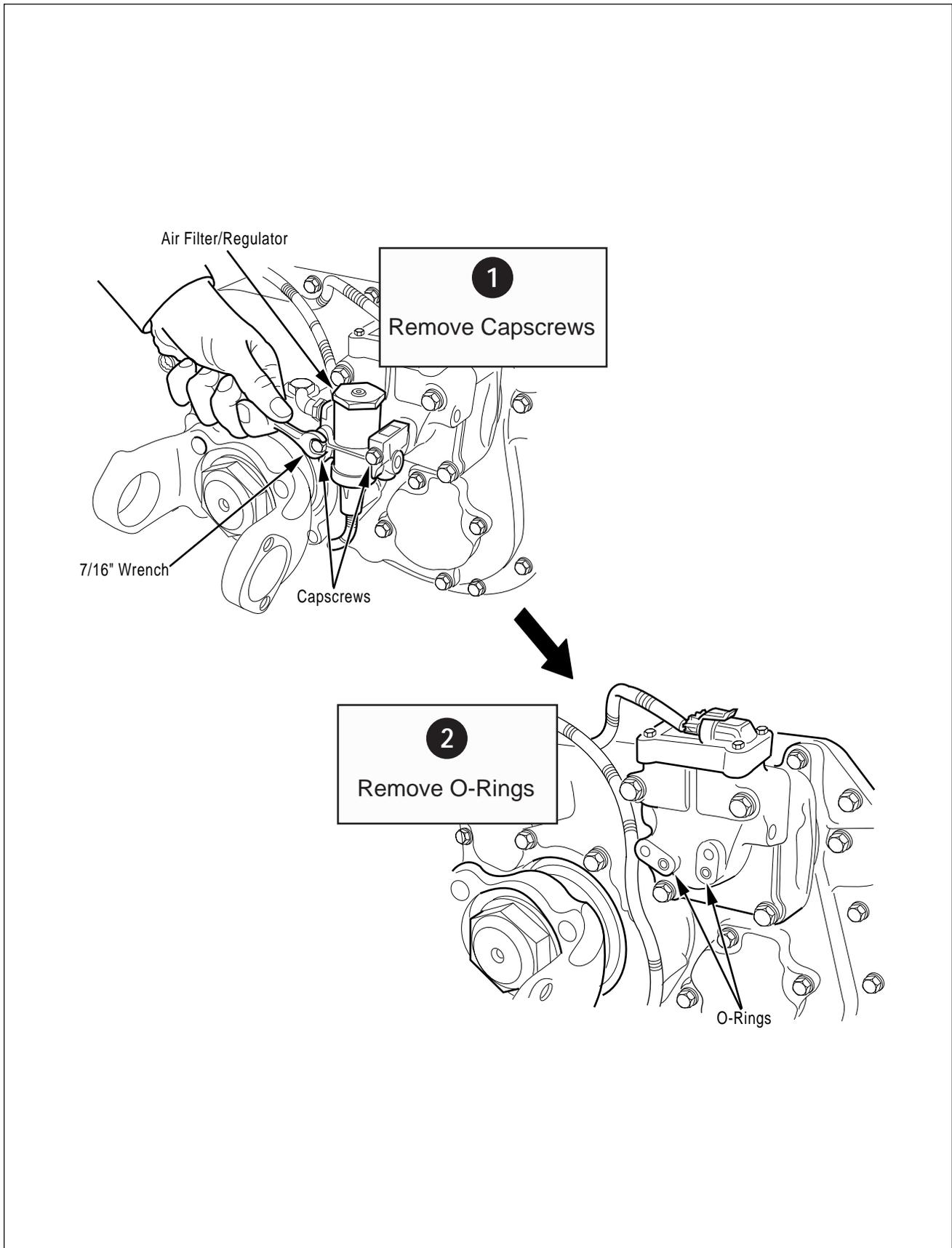
Figure 20. Air Filter/Regulator Removal
