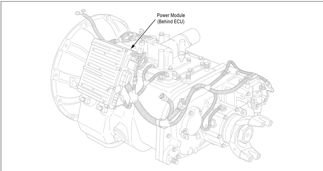
Figure 28. Power Module Location
