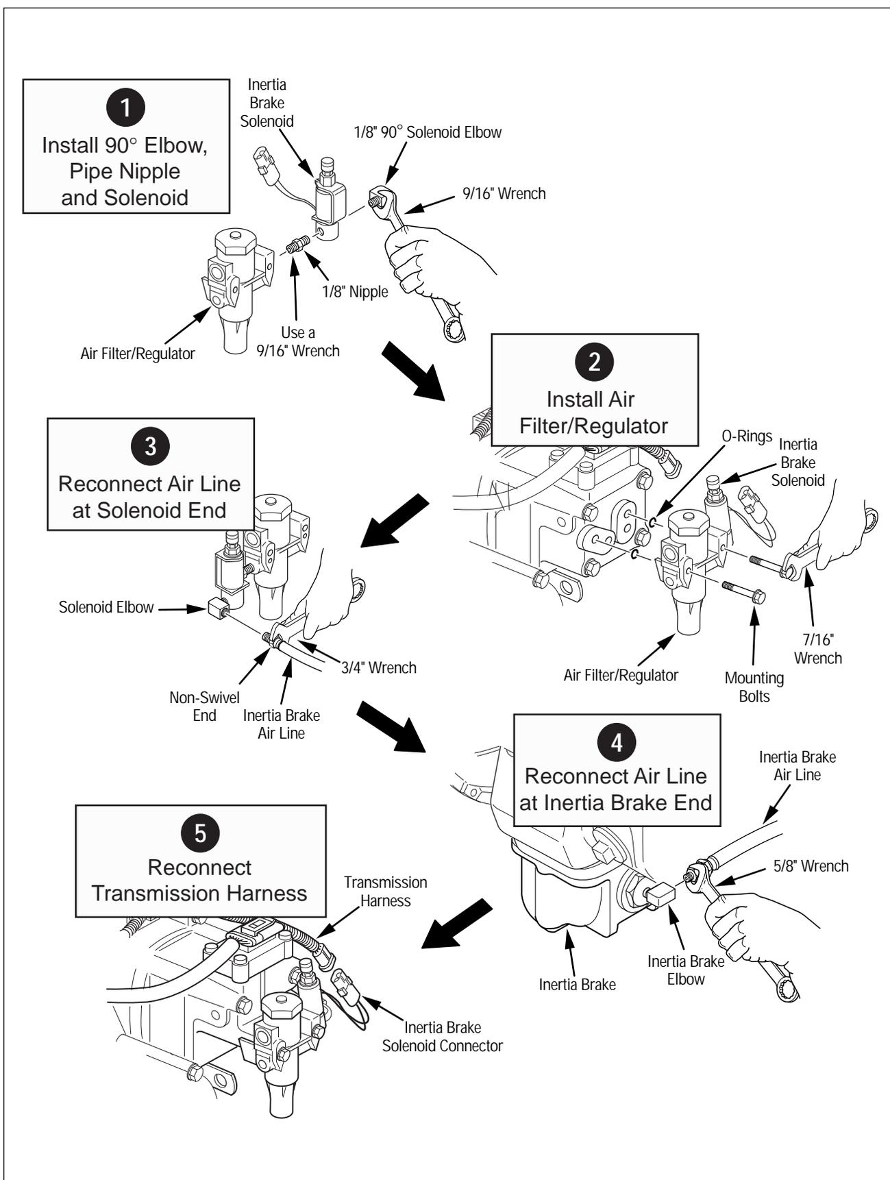
Figure 24. Inertia Brake Solenoid Installation
