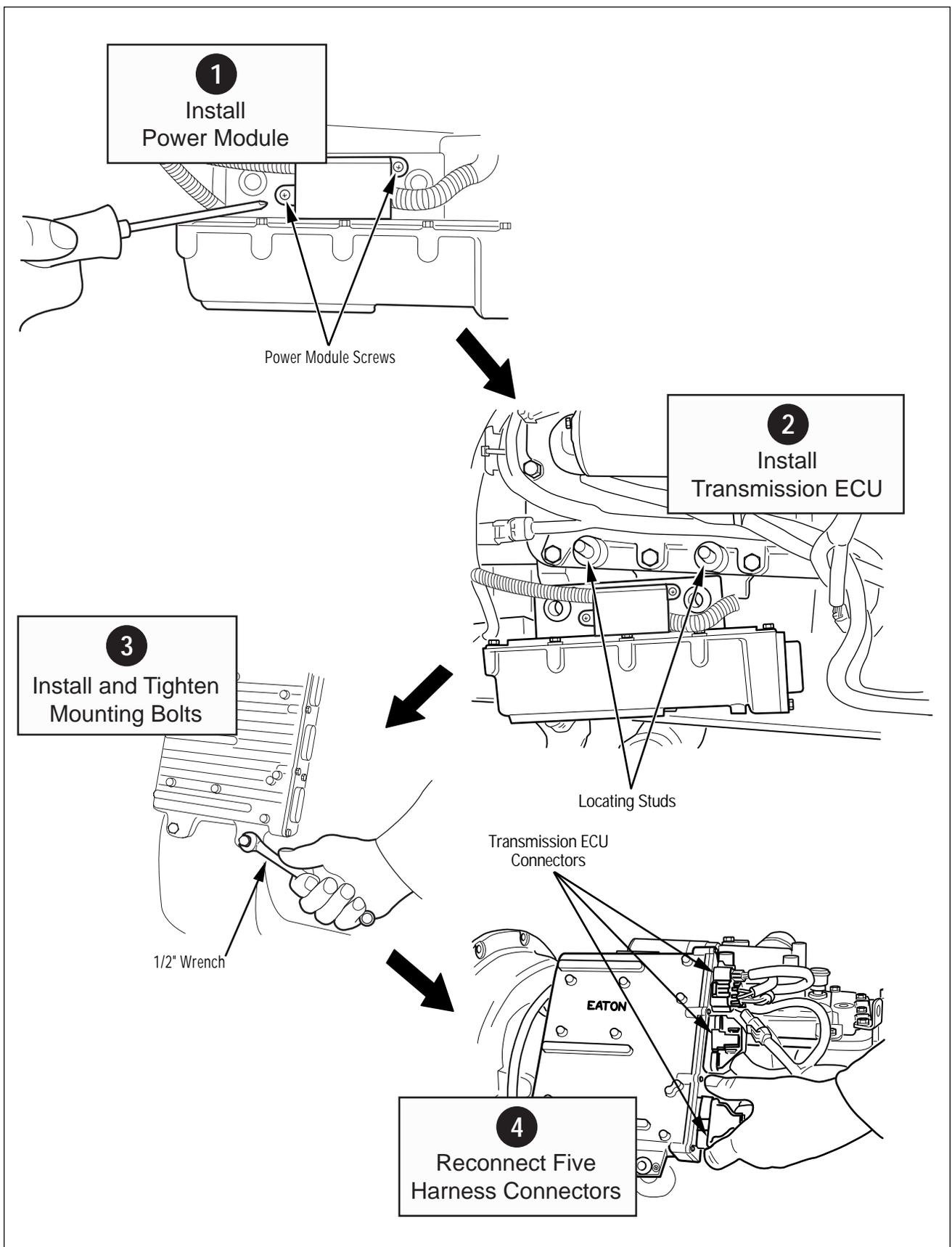
Figure 36. Transmission ECU Installation
