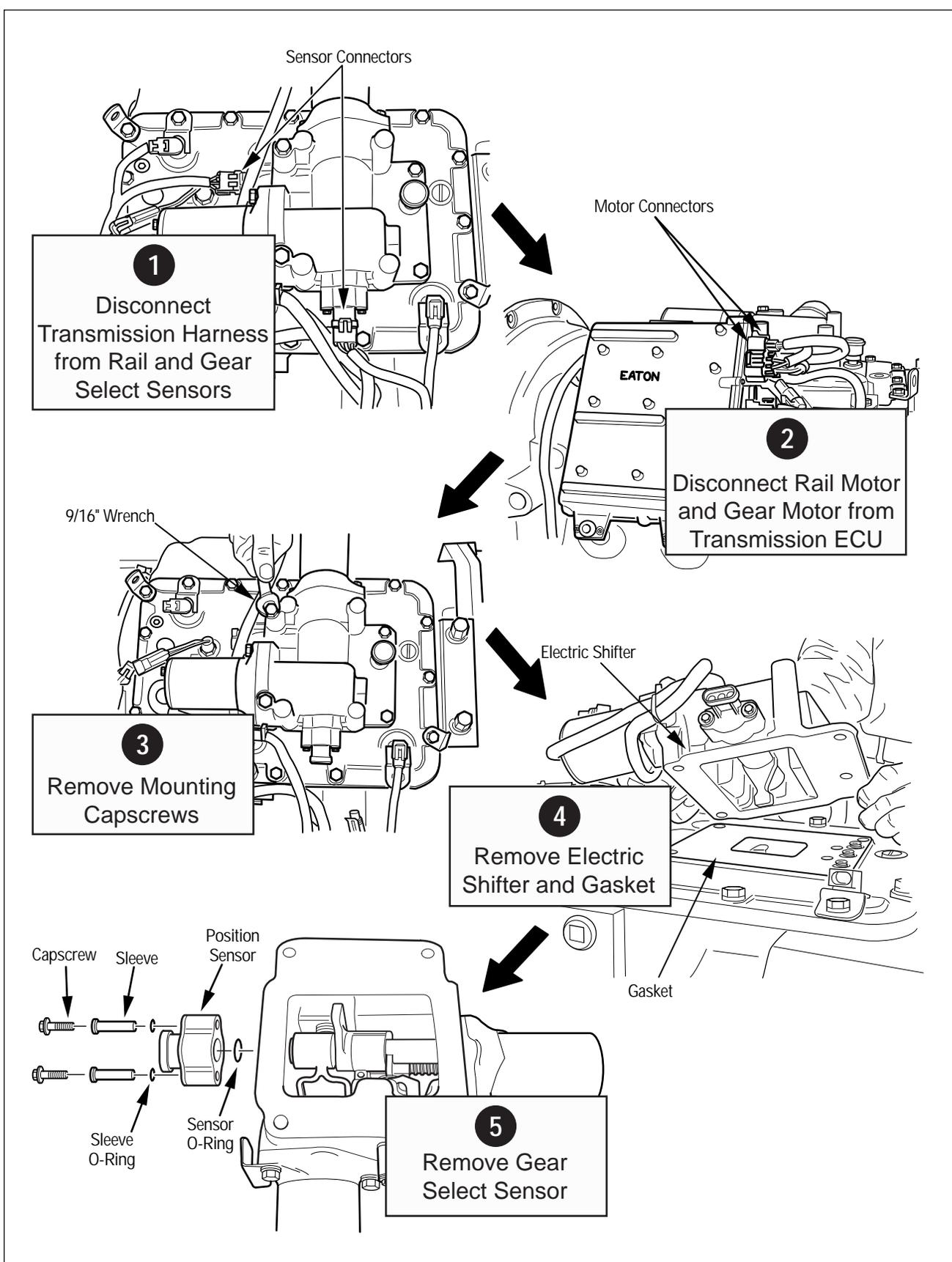
Figure 8. Gear Select Sensor Removal
