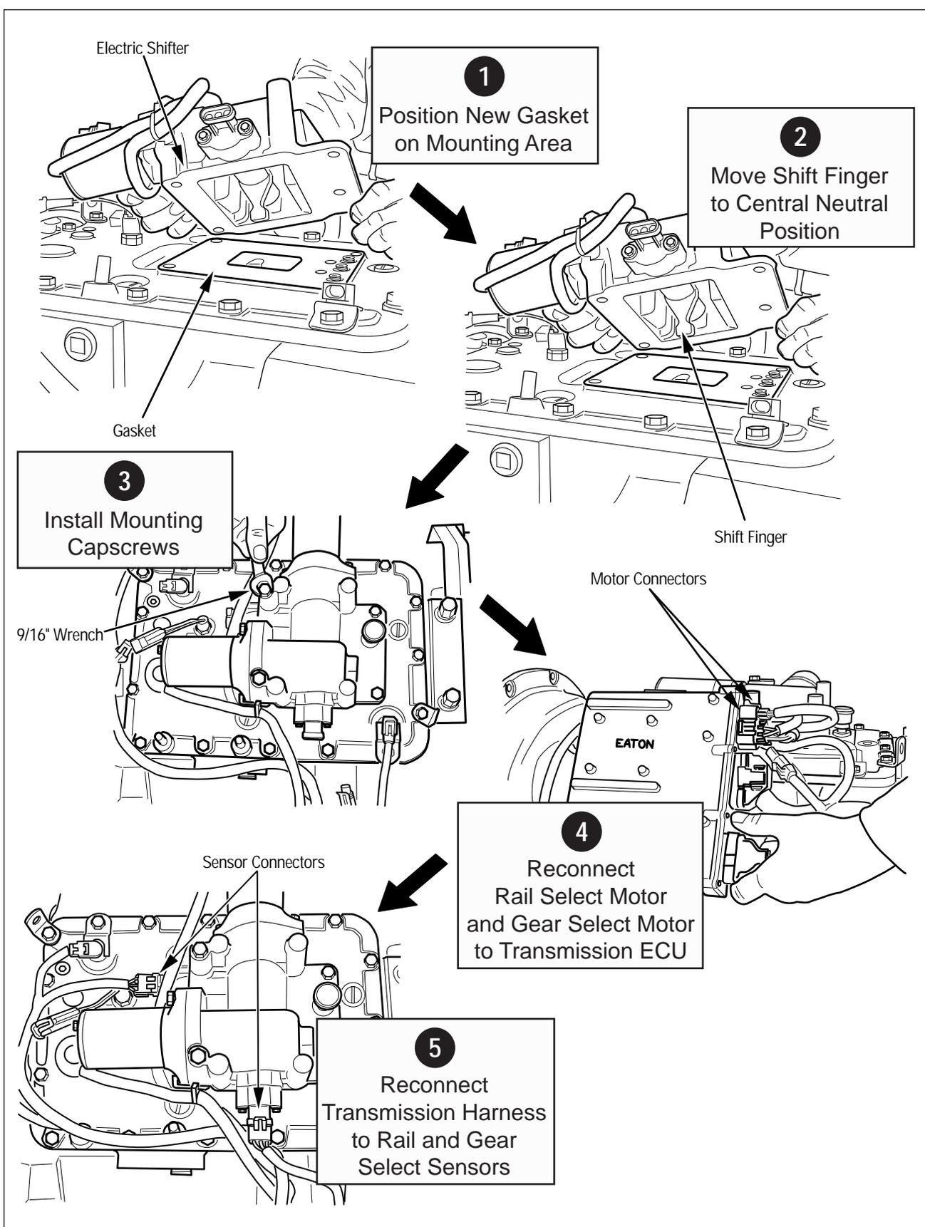
Figure 33. Electric Shifter Installation
