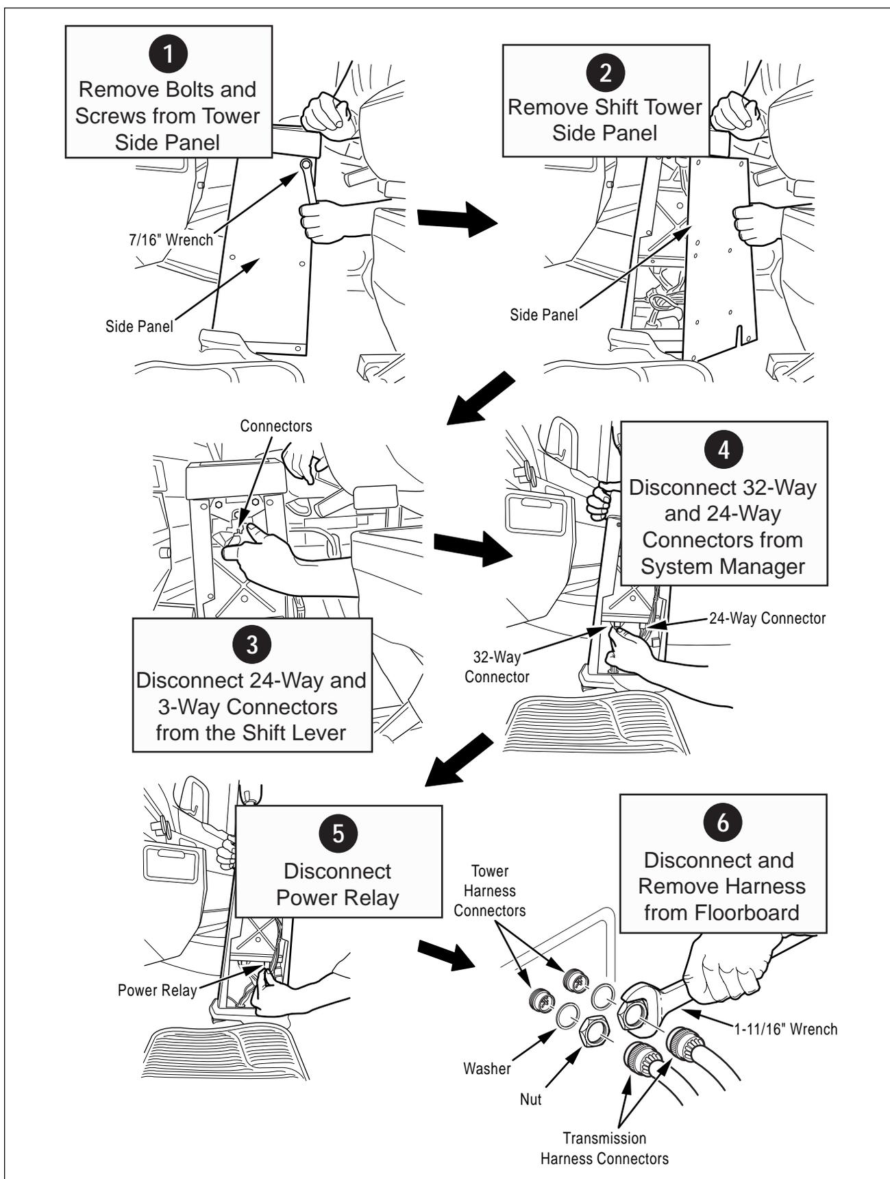
Figure 48. Tower Harness Removal
