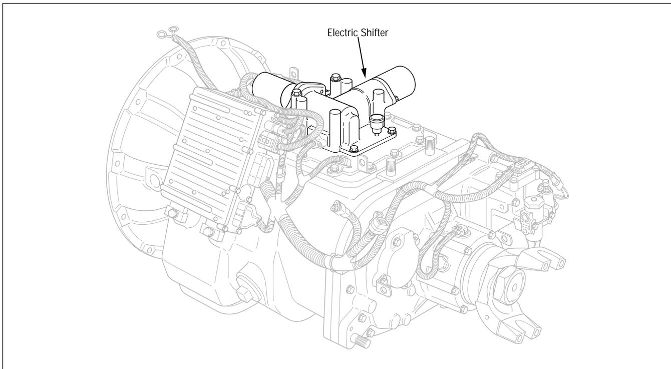
Figure 31. Electric Shifter Location
