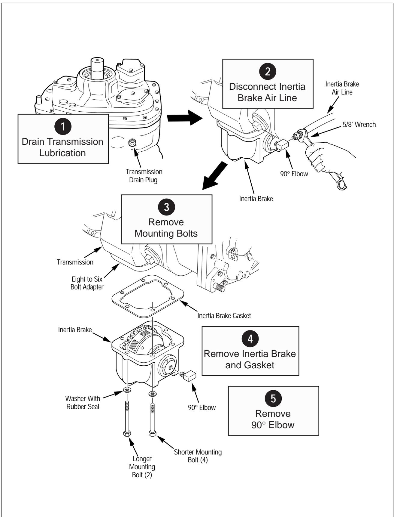
Figure 26. Inertia Brake Removal
