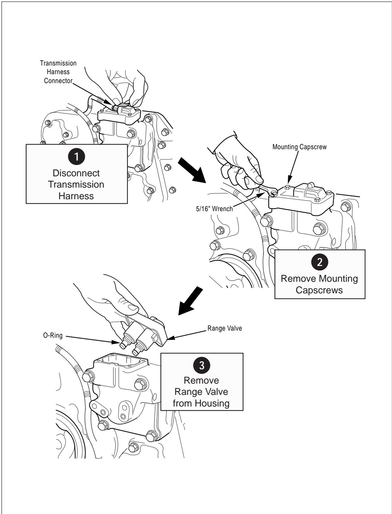
Figure 14. Range Valve Removal
