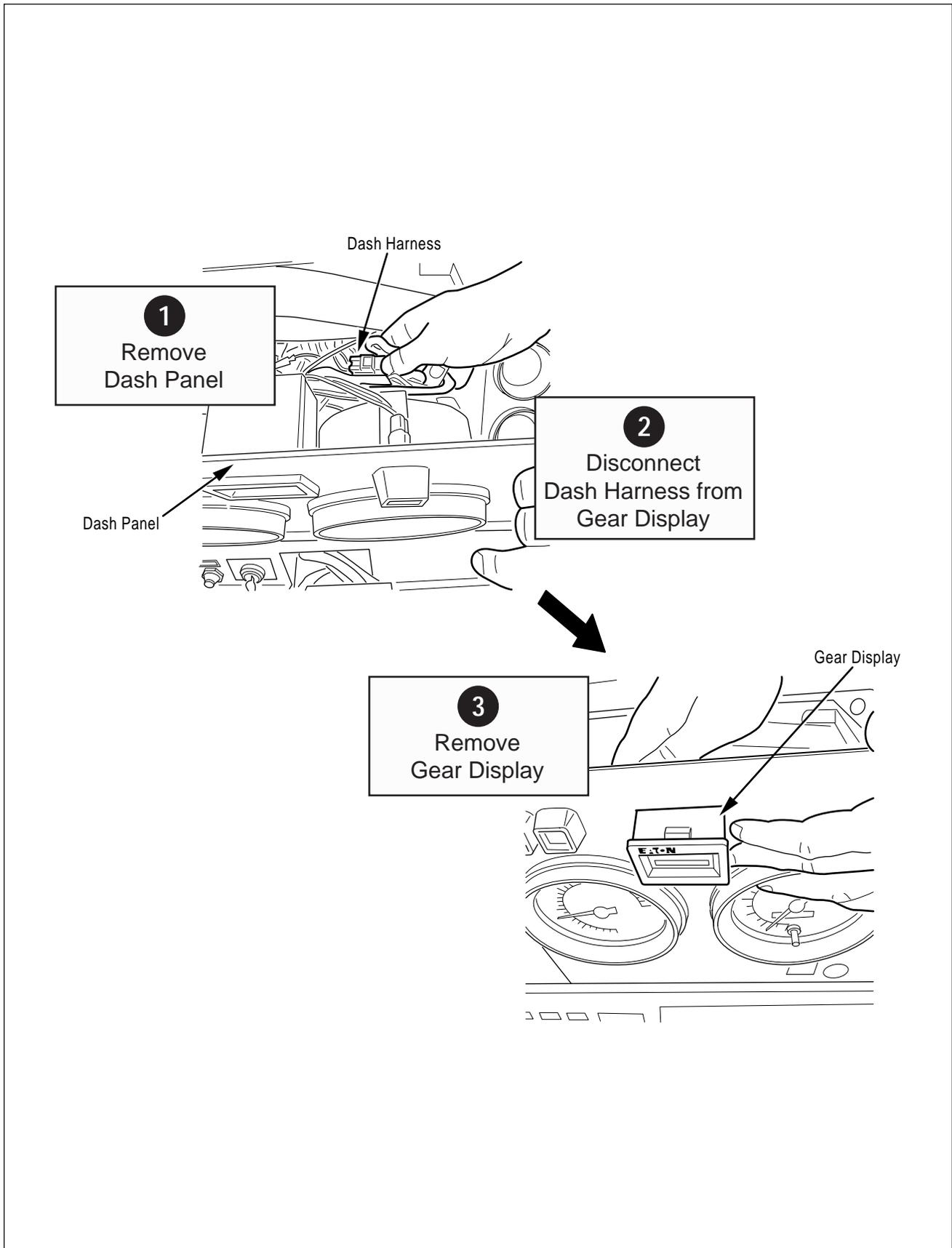
Figure 50. Gear Display Removal
