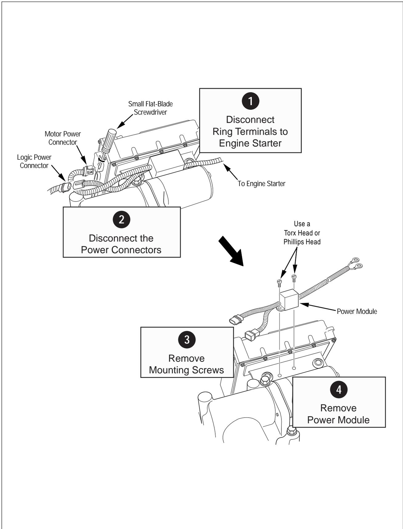
Figure 29. Power Module Removal
