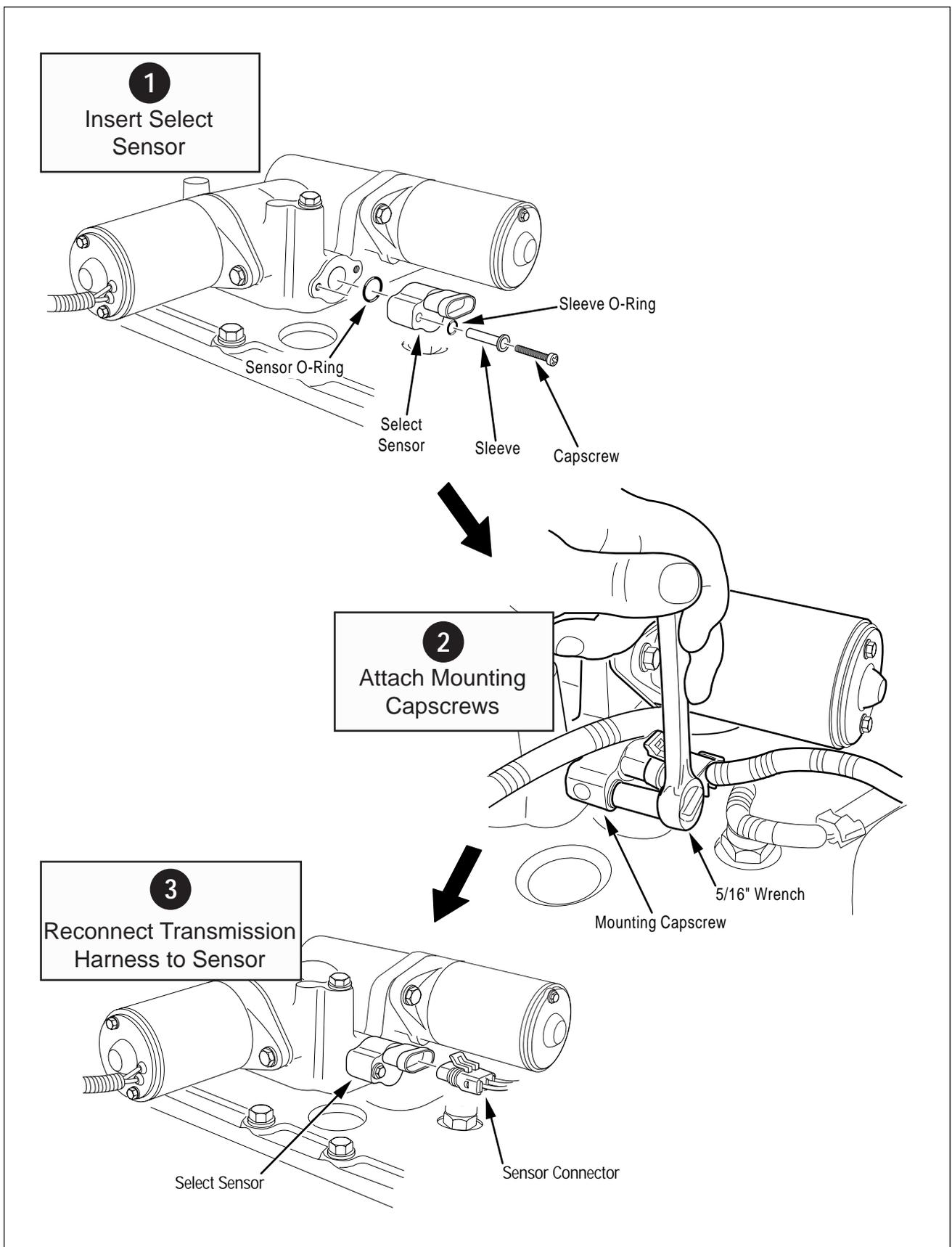
Figure 6. Rail Select Sensor Installation
