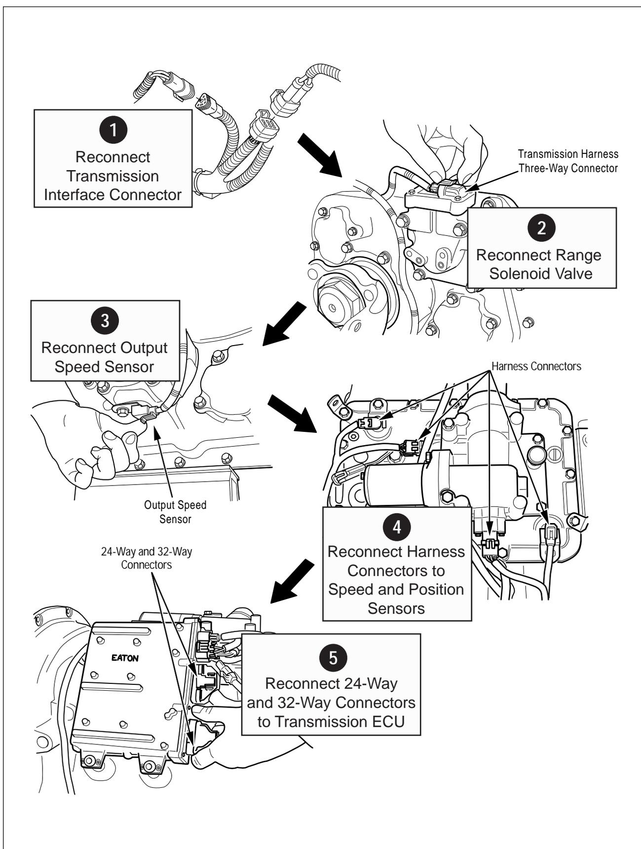
Figure 39. Transmission Harness Installation
