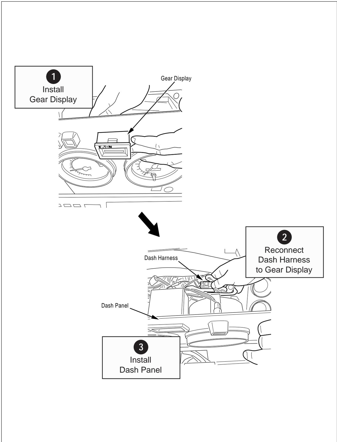
Figure 51. Gear Display Installation
