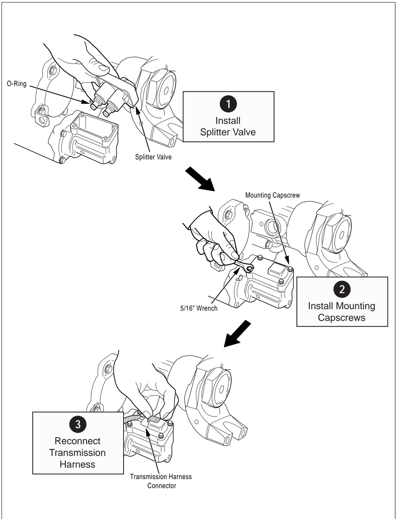
Figure 18. Splitter Valve Installation
