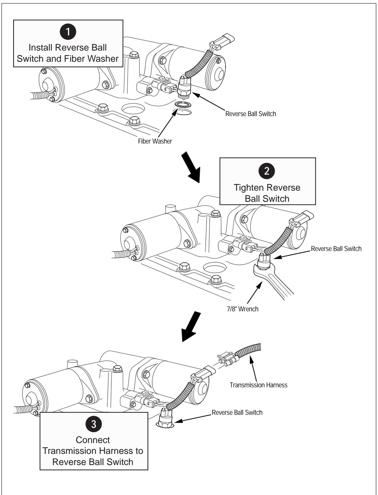
Figure 3. Reverse Ball Switch Installation
