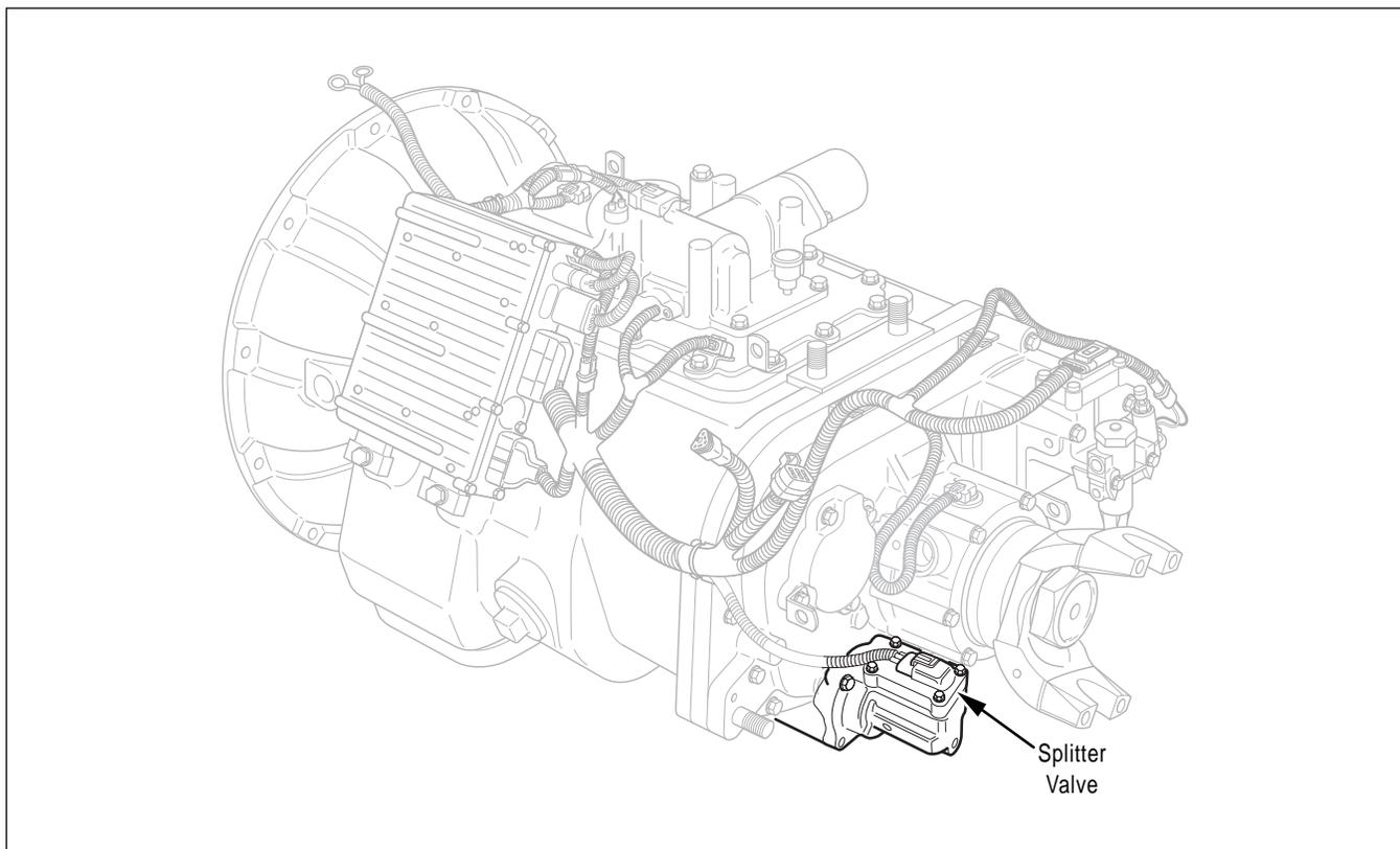
Figure 16. Splitter Valve Location
