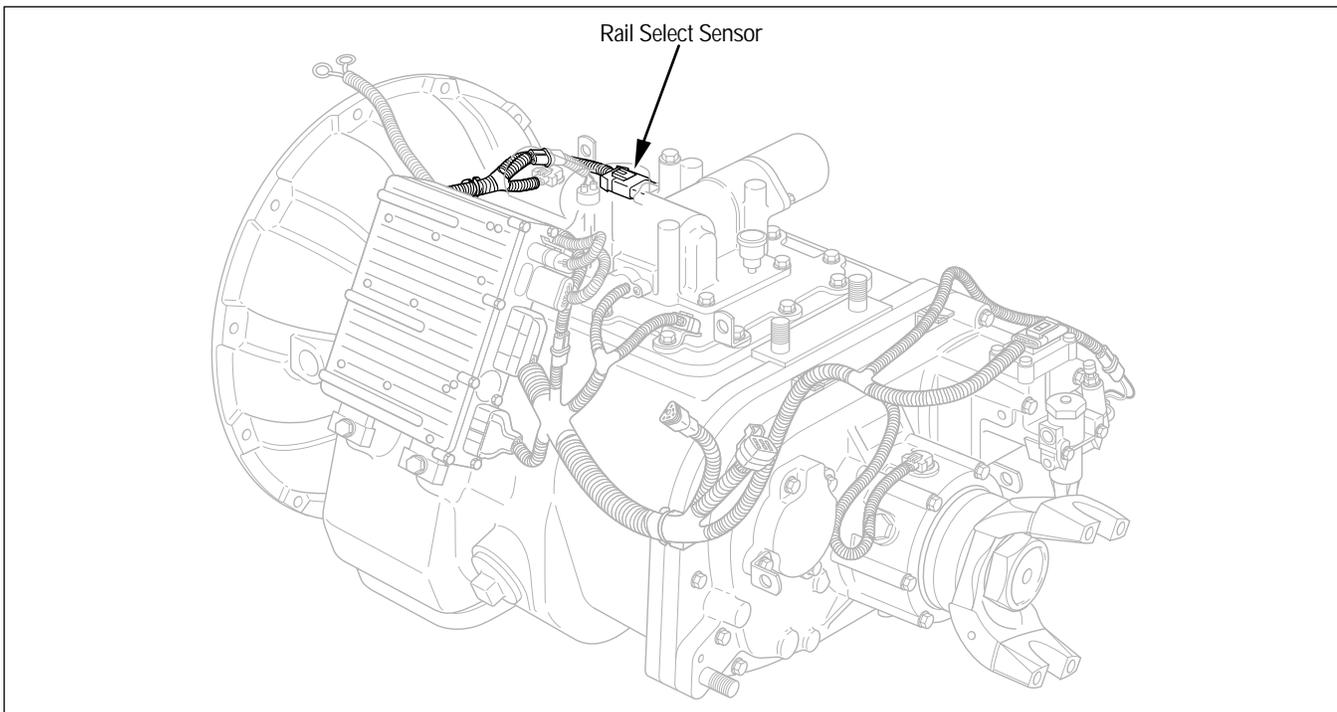
Figure 4. Rail Select Sensor Location
