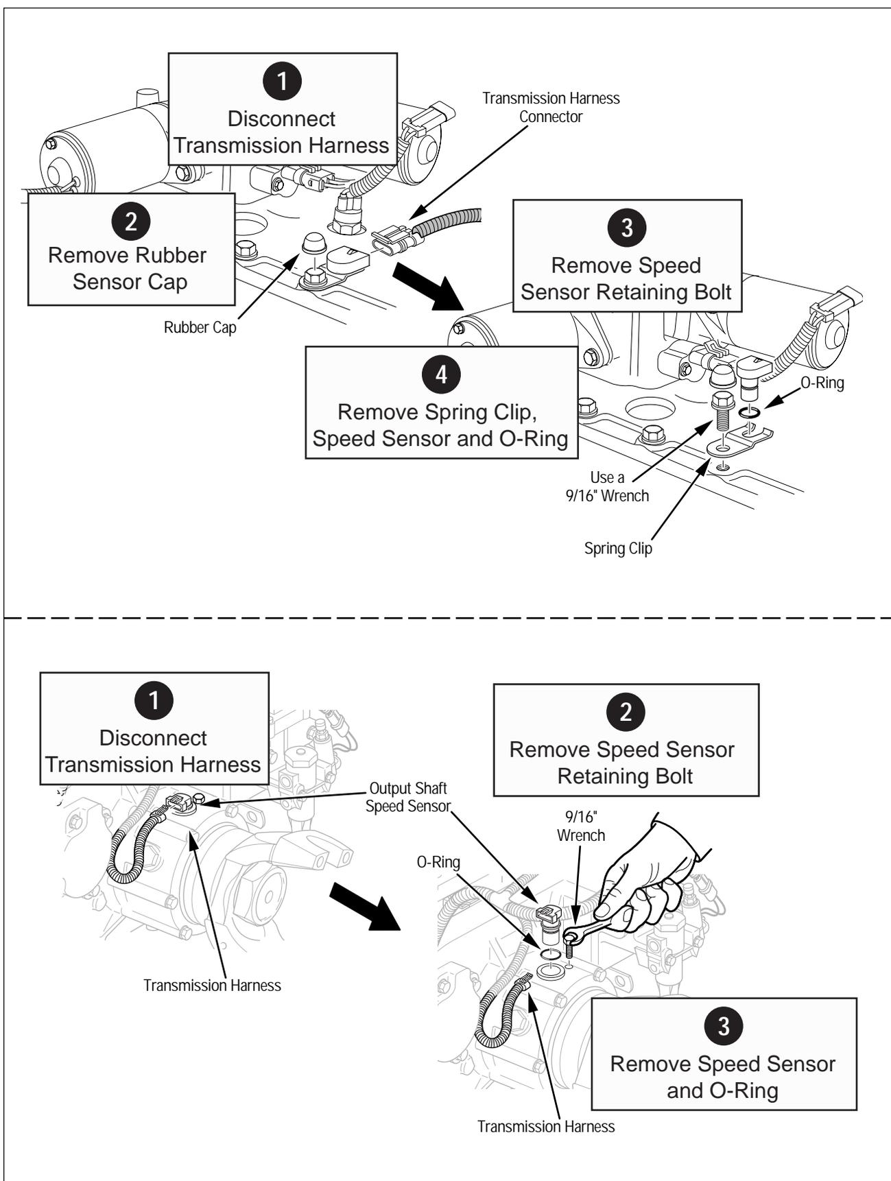
Figure 11. Input/Main/Output Speed Sensor Removal
