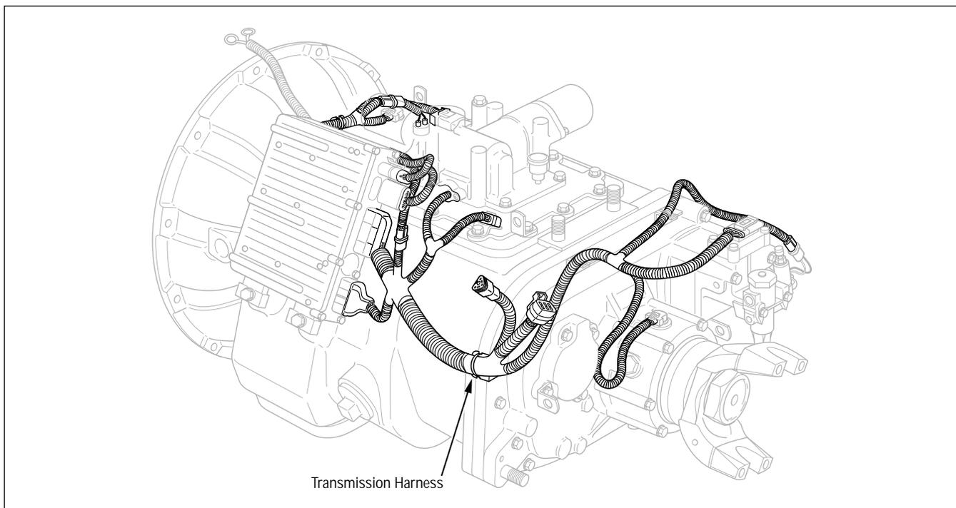
Figure 37. Transmission Harness Location
