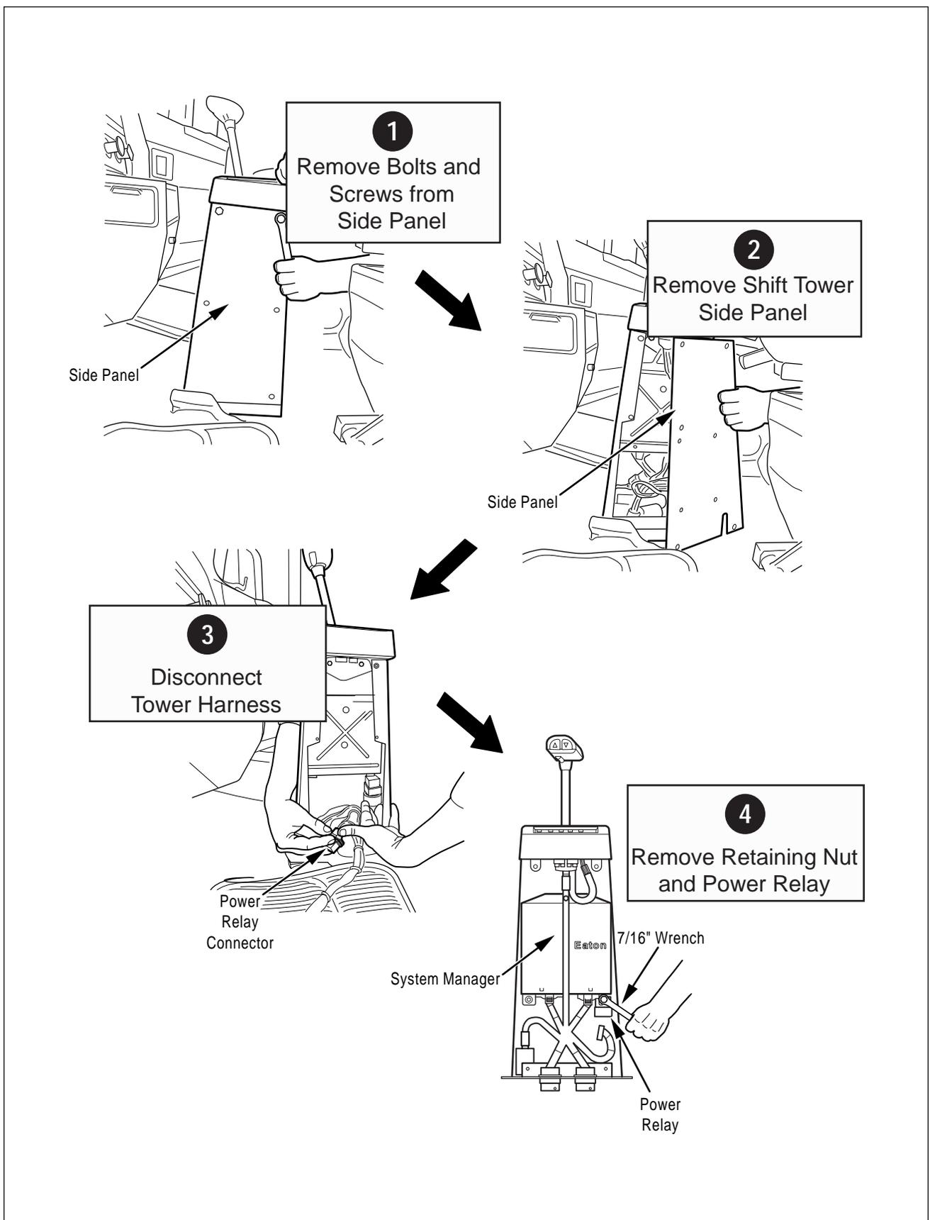
Figure 42. Power Relay Removal
