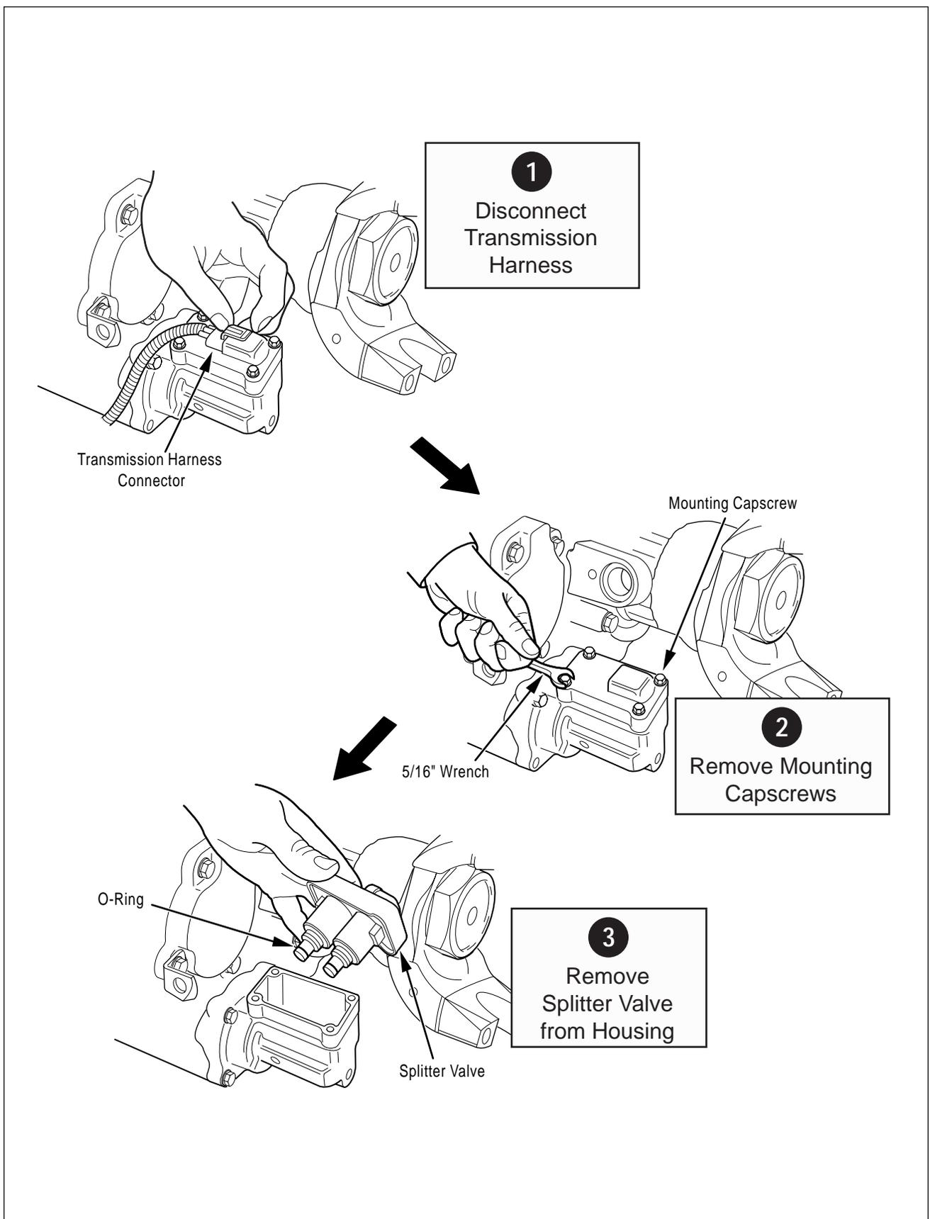
Figure 17. Splitter Valve Removal
