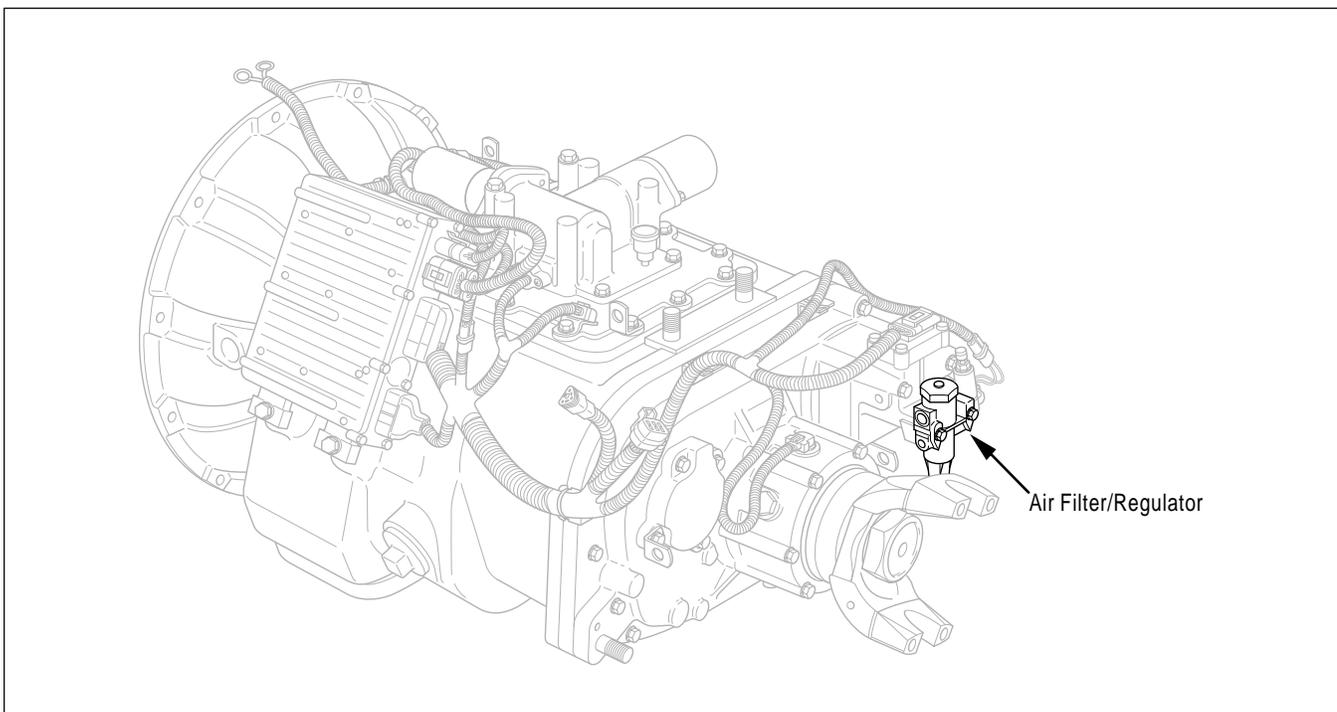
Figure 19. Air Filter/Regulator Location
