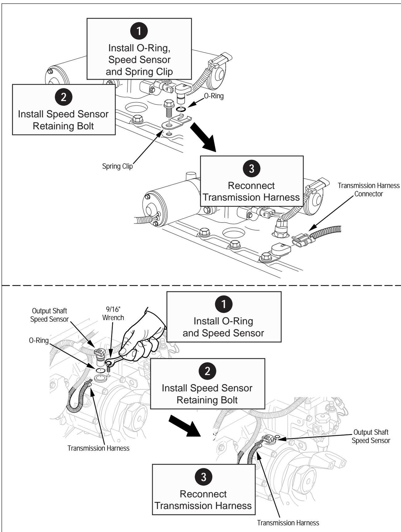
Figure 12. Input/Main/Output Speed Sensor Installation
