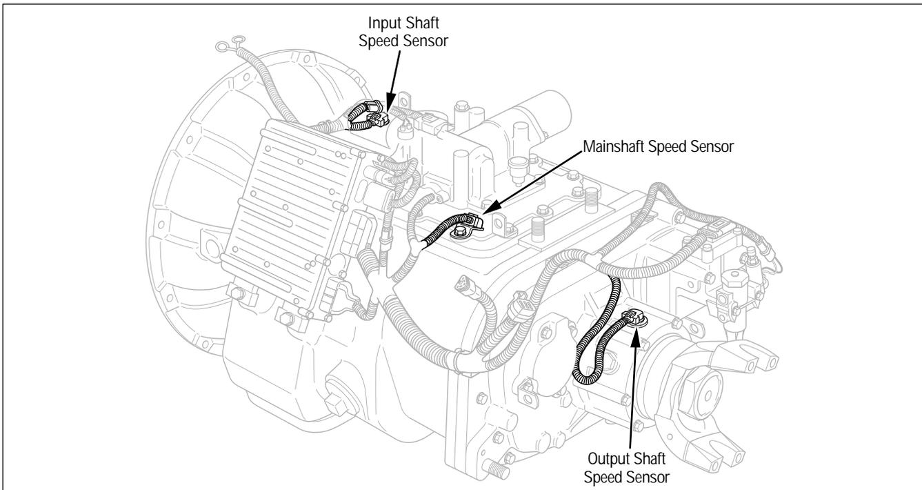
Figure 10. Input/Main/Output Shaft Speed Sensor Locations
