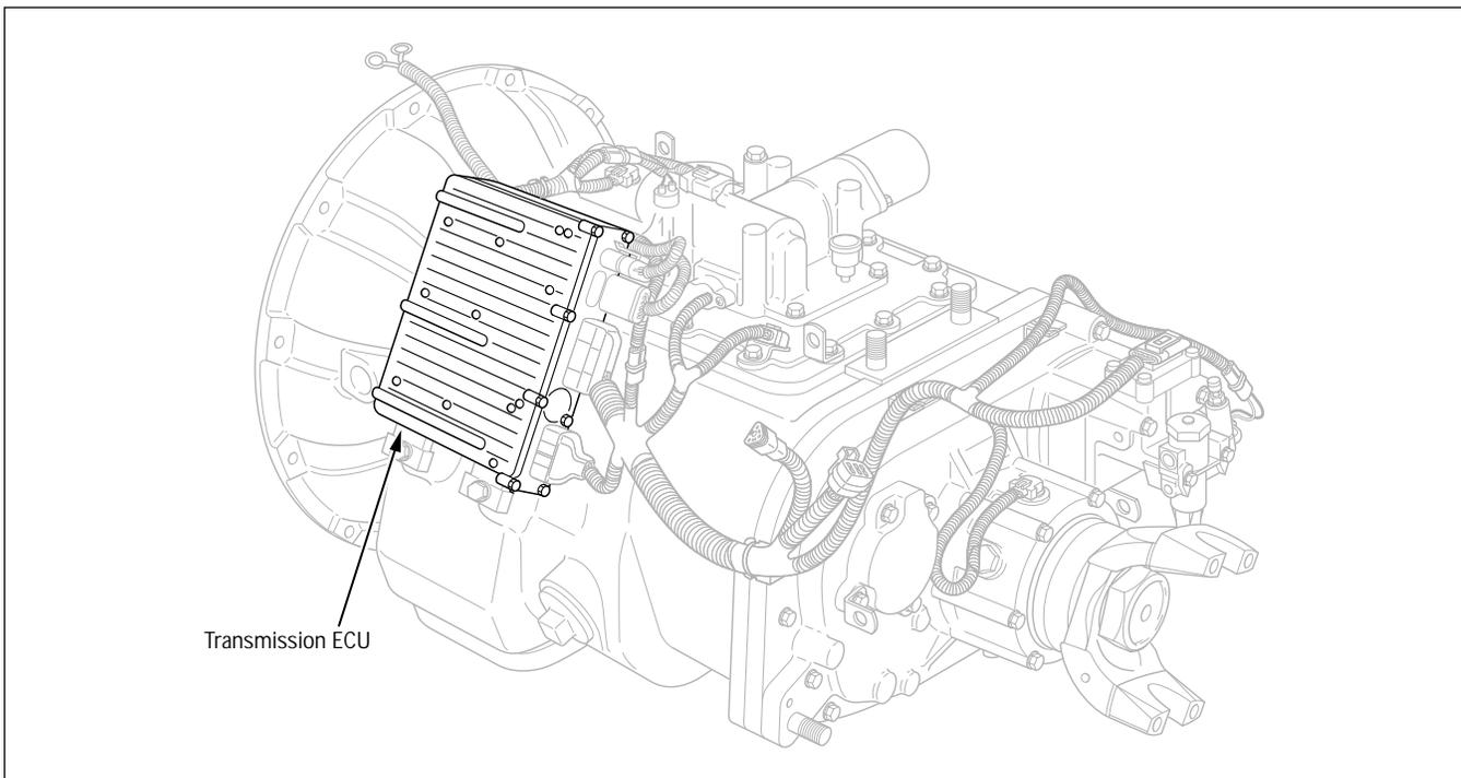
Figure 34. Transmission ECU Location
