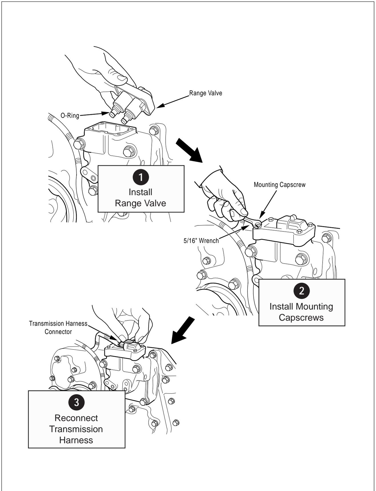
Figure 15. Range Valve Installation
