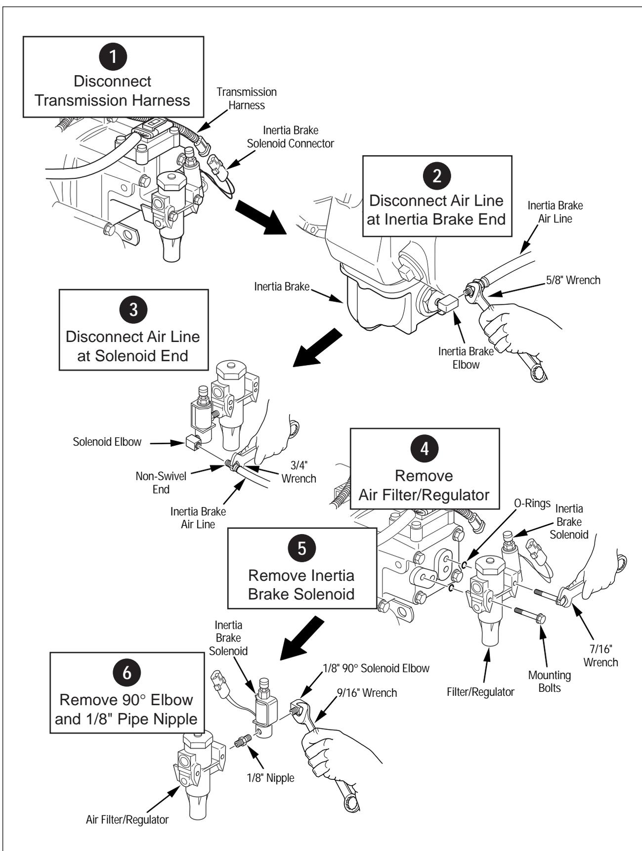
Figure 23. Inertia Brake Solenoid Removal
