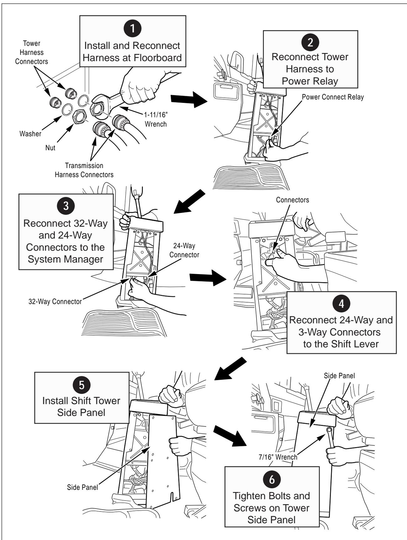
Figure 49. Tower Harness Installation
