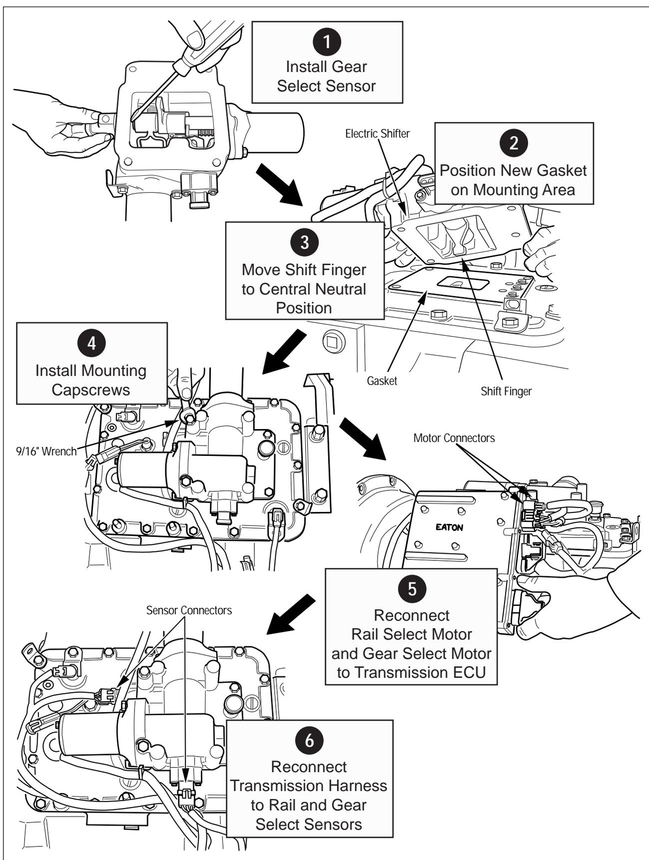
Figure 9. Gear Select Sensor Installation
