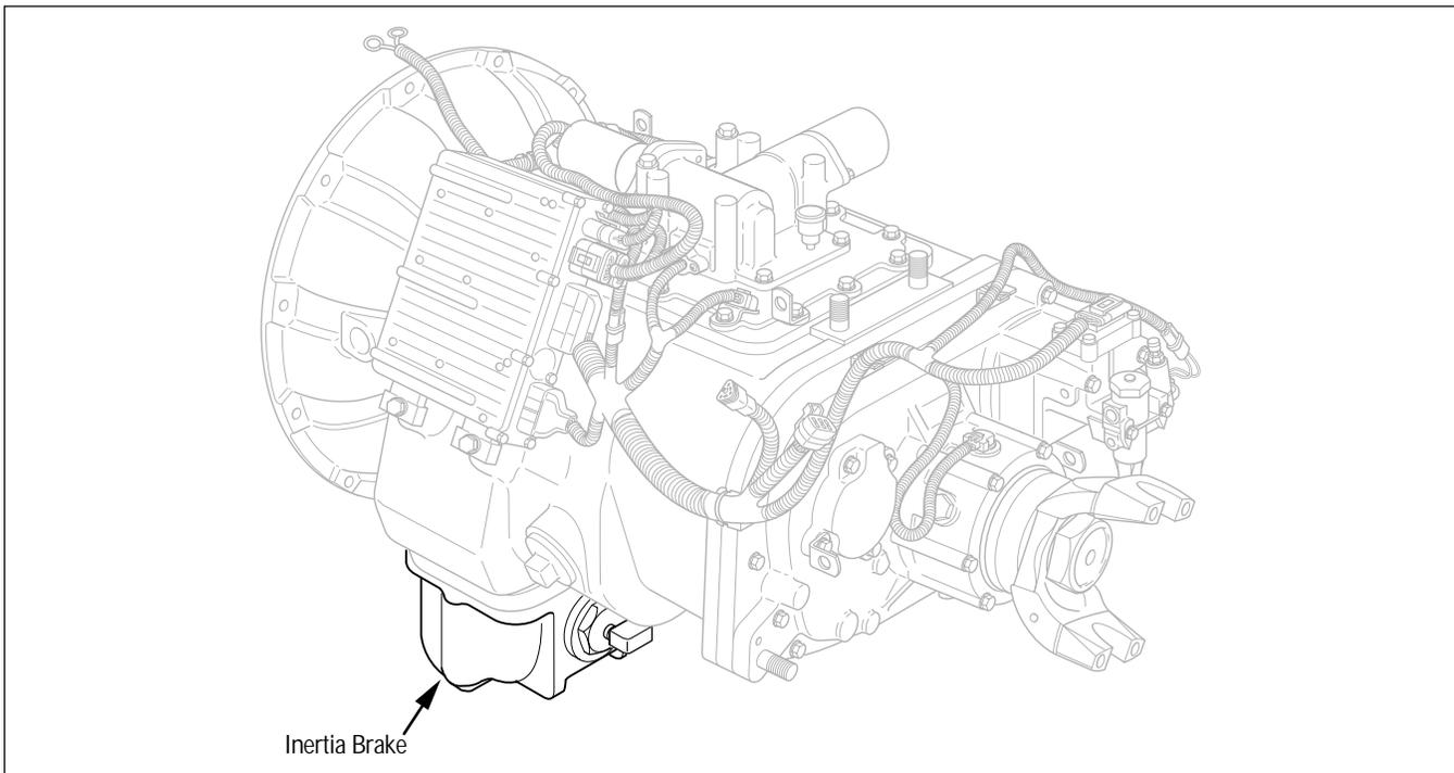
Figure 25. Inertia Brake Location
