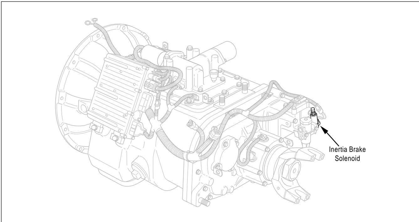
Figure 22. Inertia Brake Solenoid Location
