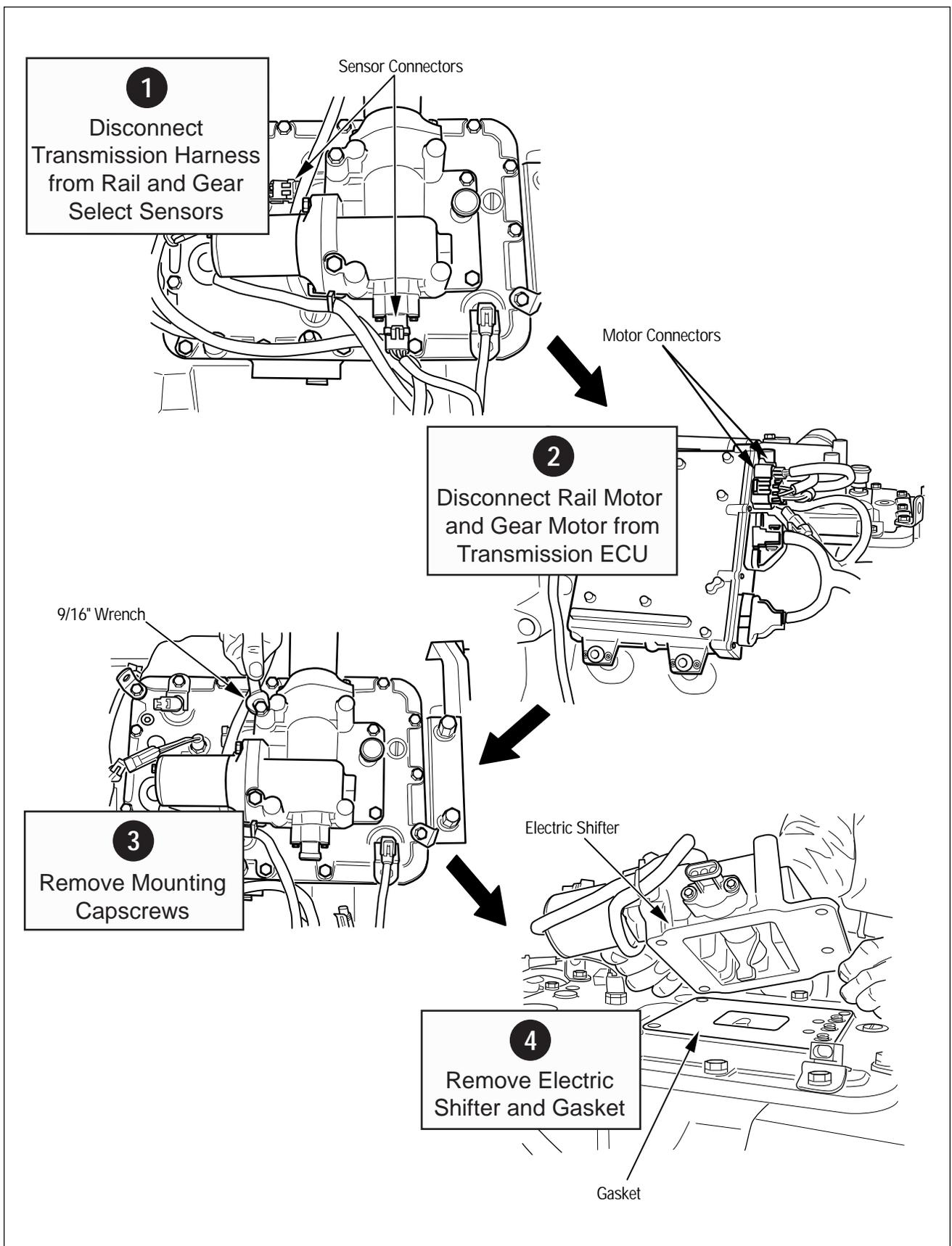
Figure 32. Electric Shifter Removal
