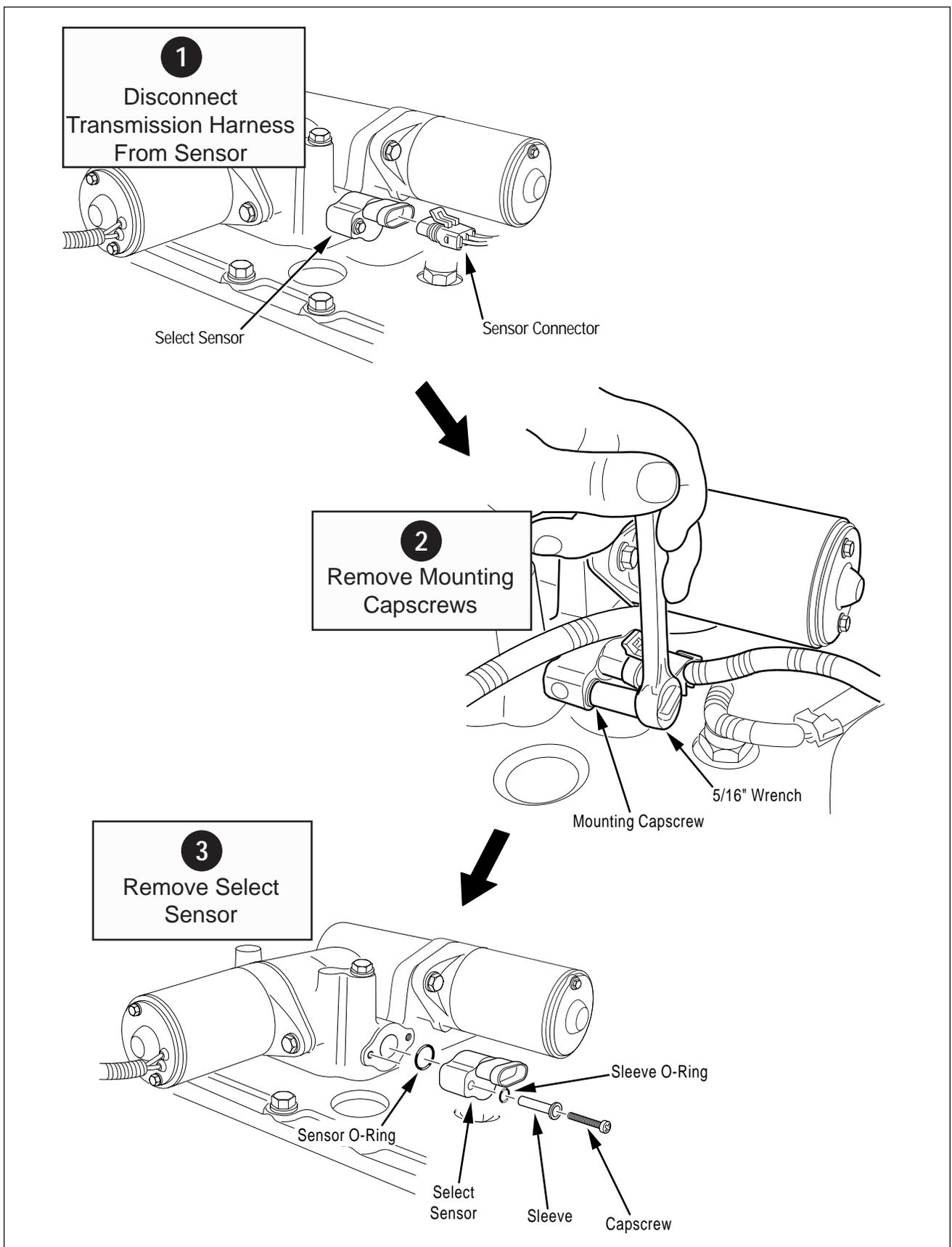
Figure 5. Rail Select Sensor Removal
