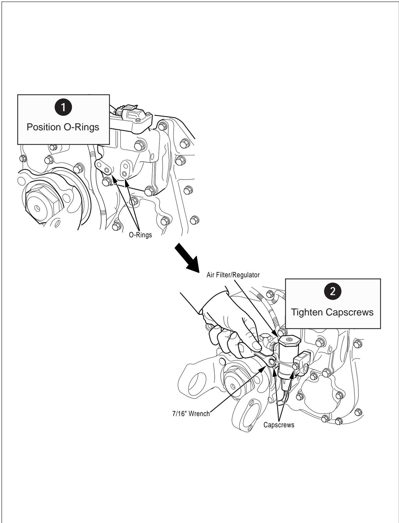
Figure 21. Air Filter/Regulator Installation
