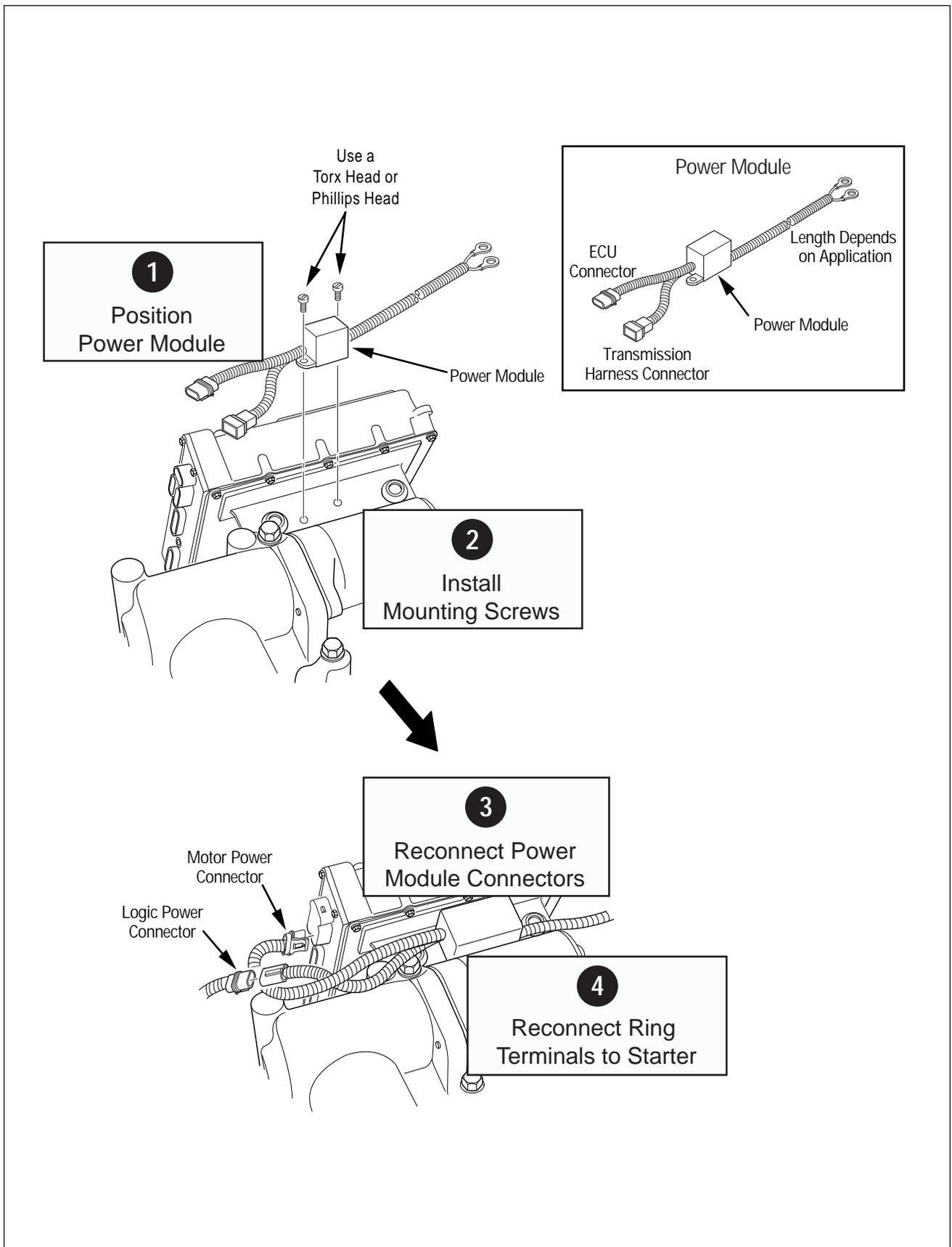
Figure 30. Power Module Installation
