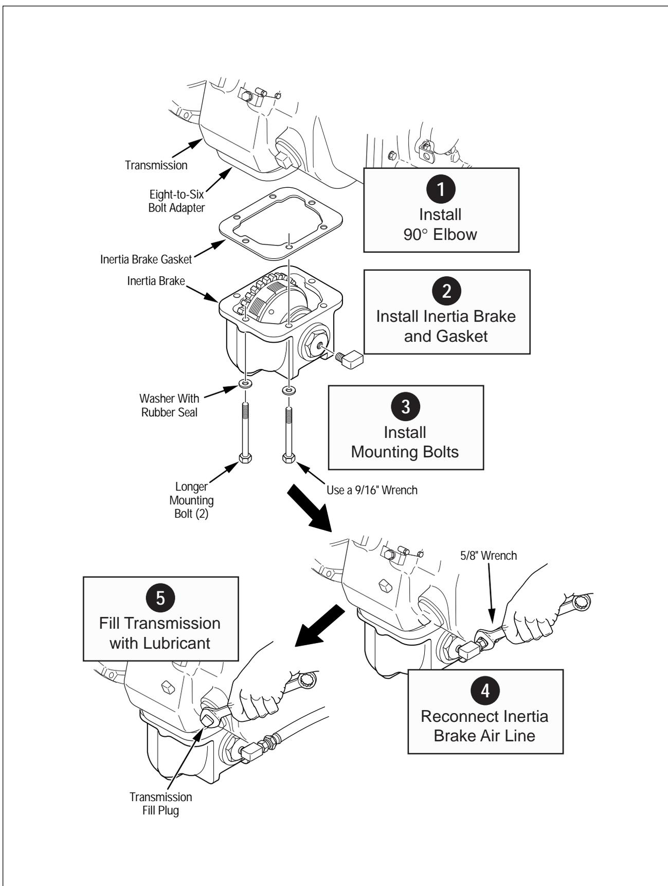
Figure 27. Inertia Brake Installation
