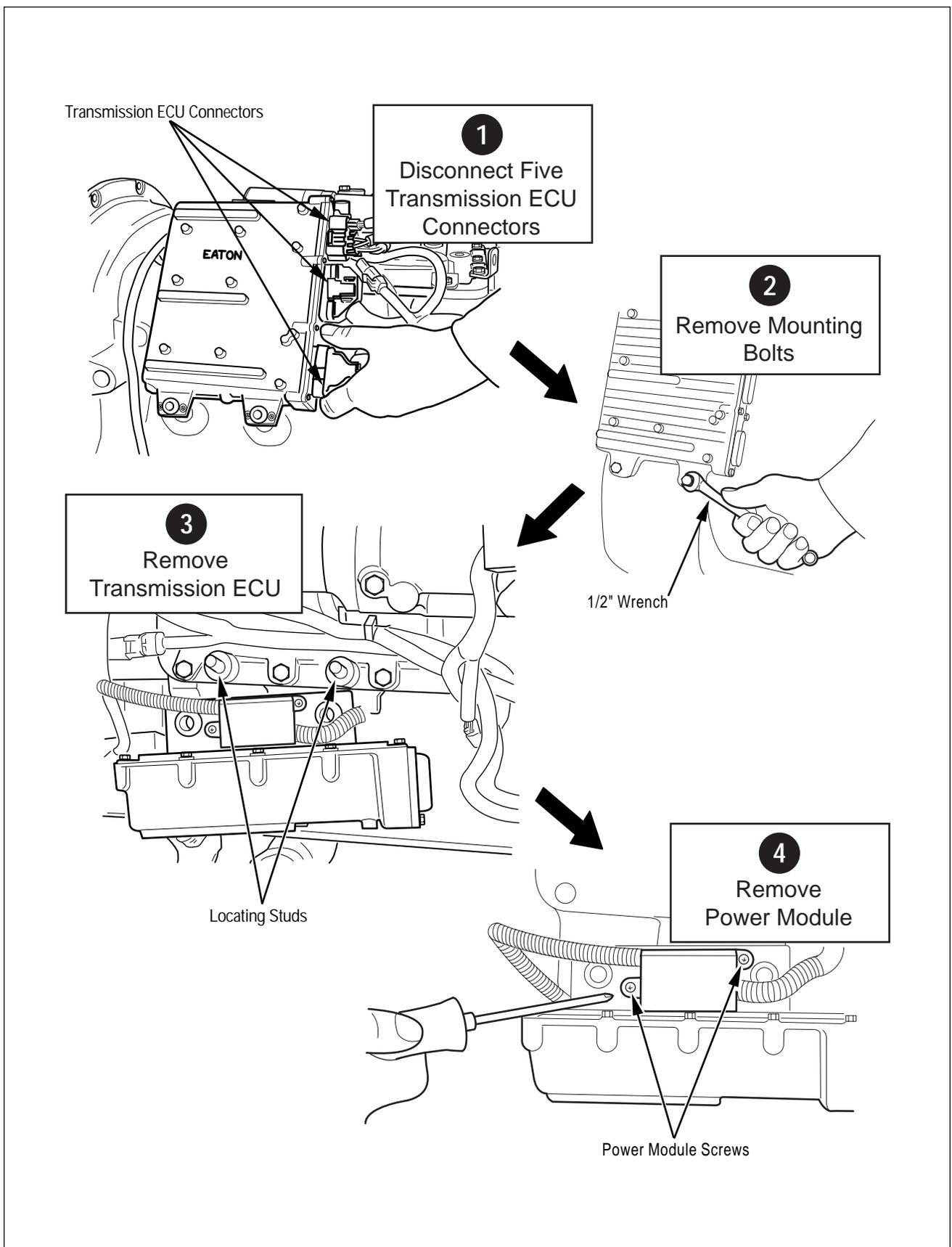
Figure 35. Transmission ECU Removal
