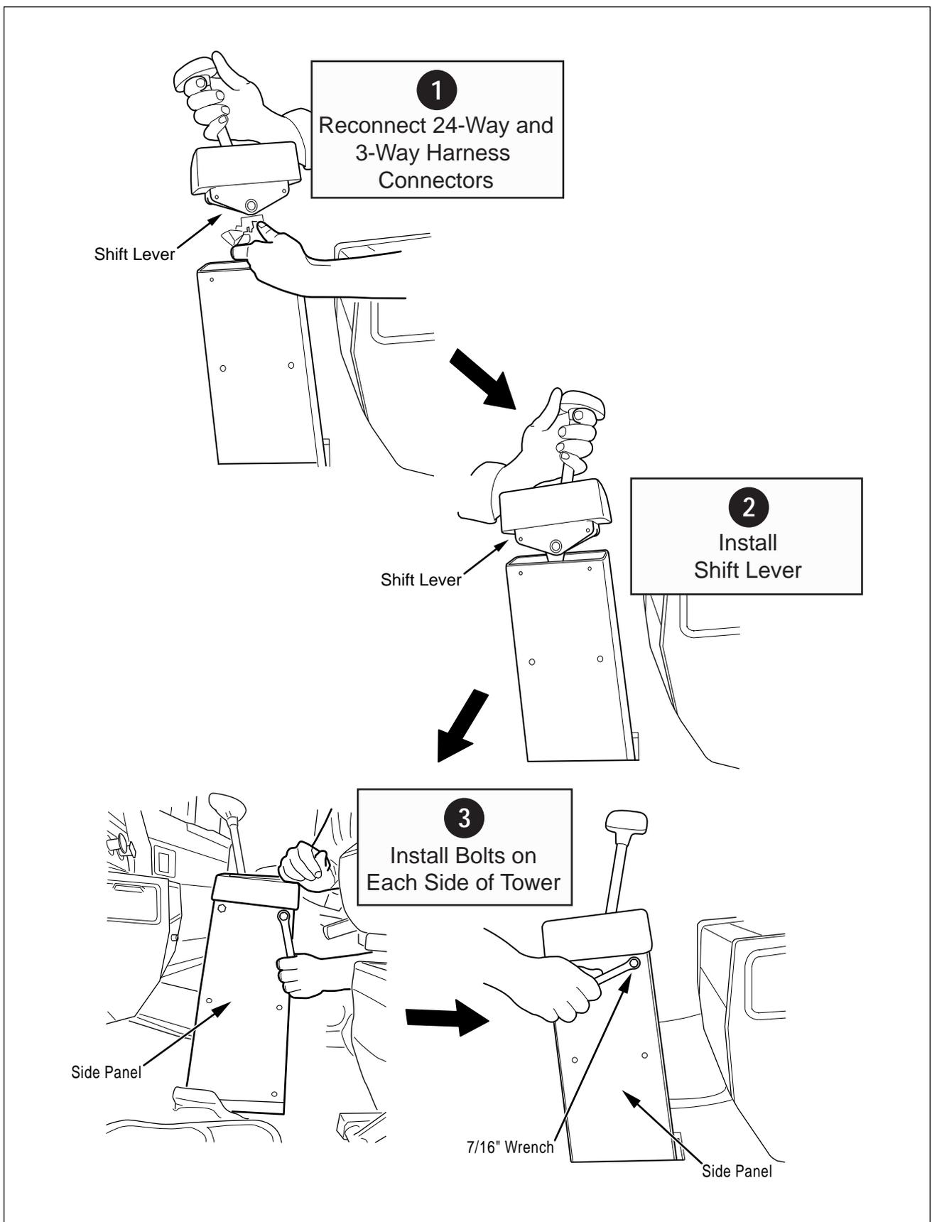
Figure 41. Shift Lever Installation
