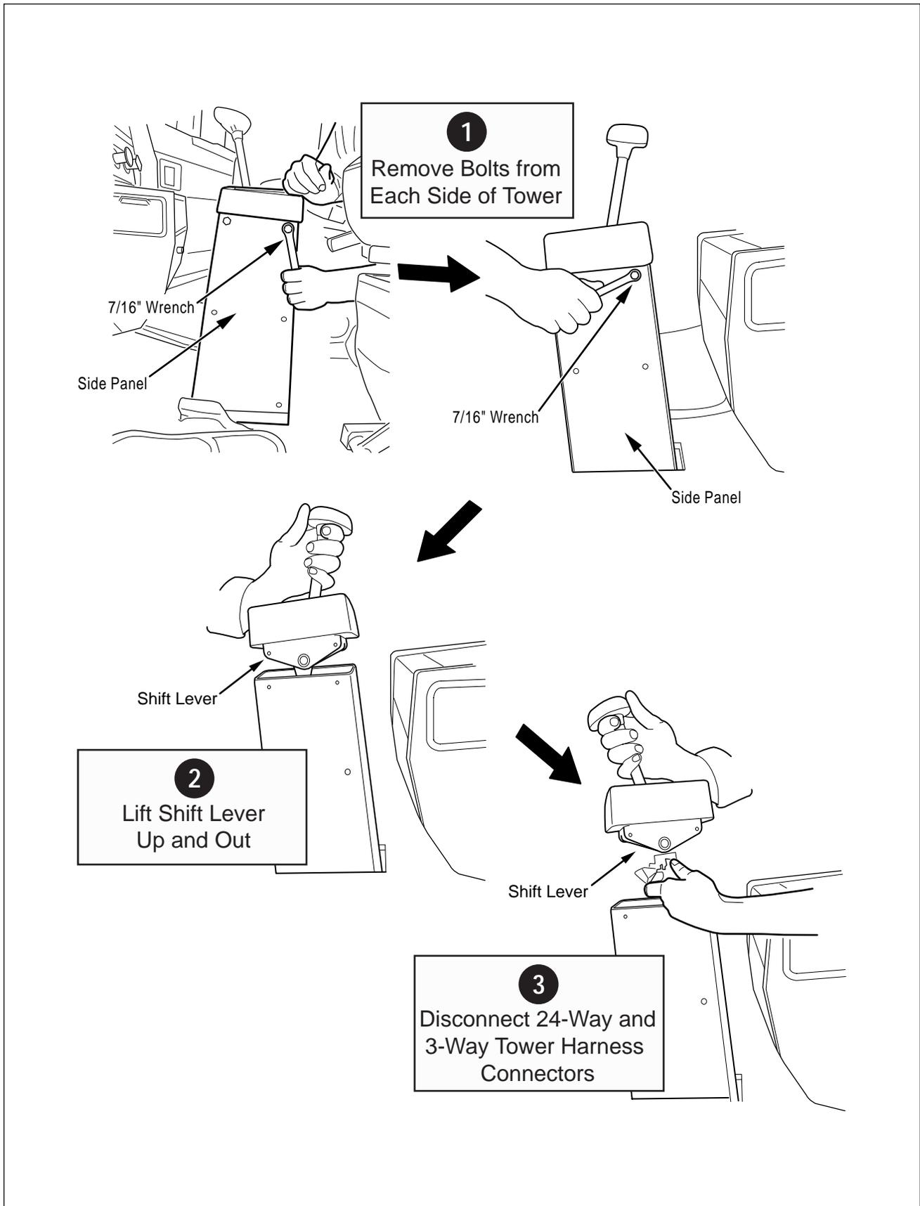
Figure 40. Shift Lever Removal
