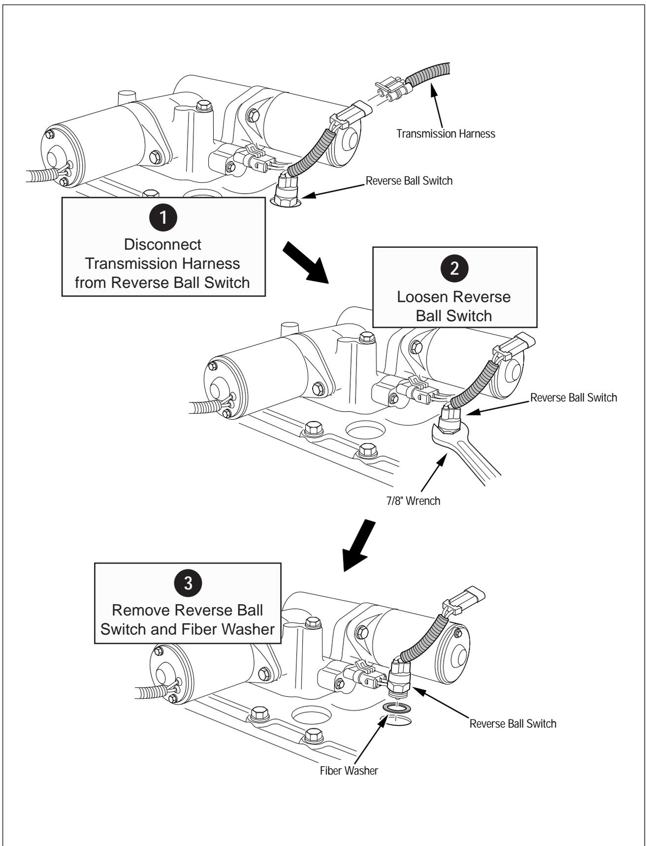
Figure 2. Reverse Ball Switch Removal
