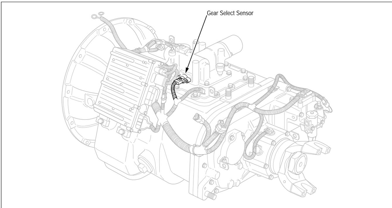
Figure 7. Gear Select Sensor Location
