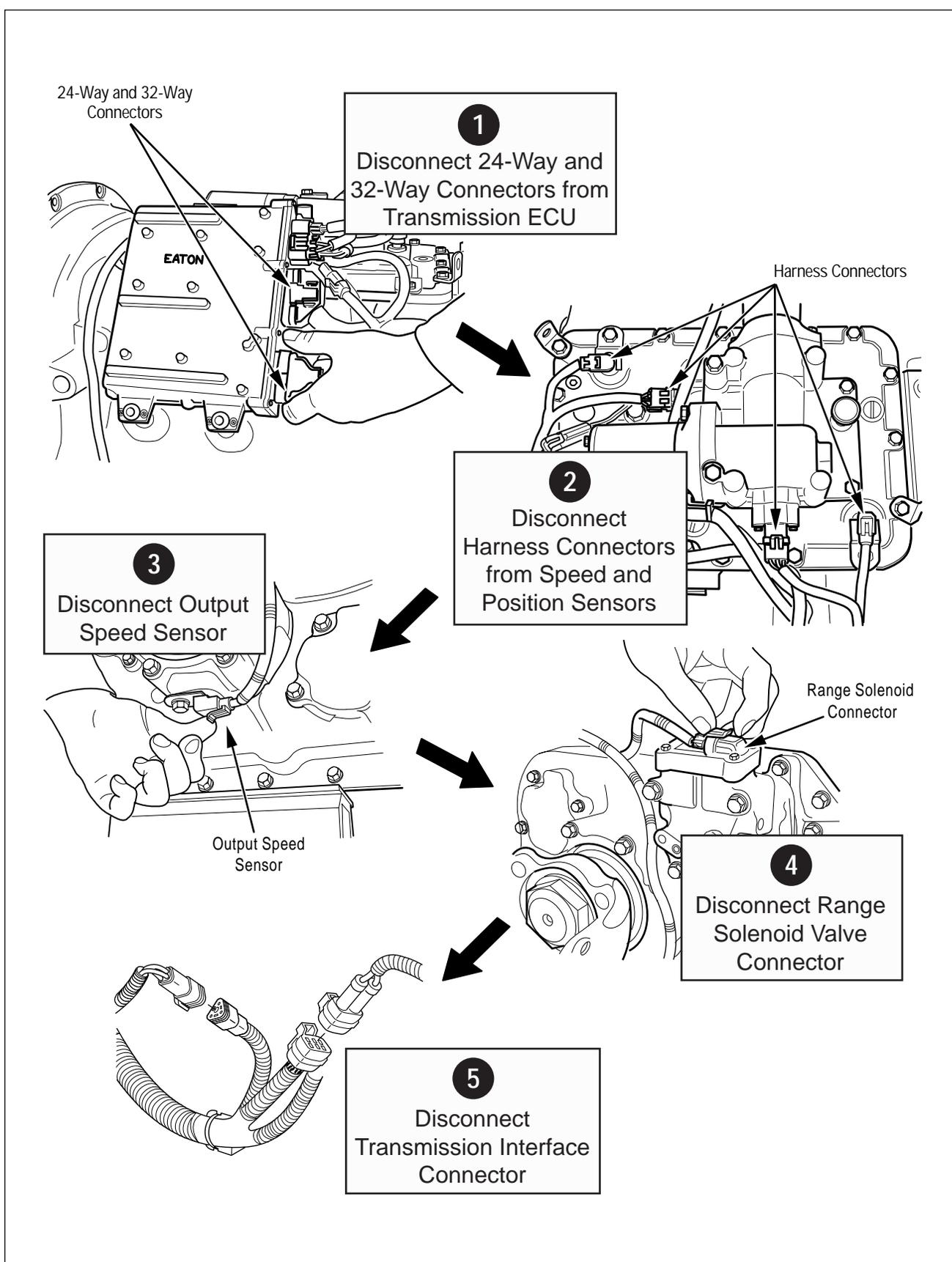
Figure 38. Transmission Harness Removal
