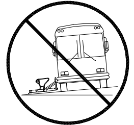
FIGURE 2-1: VEHICLE INCLINED DUE TO SLOPE
