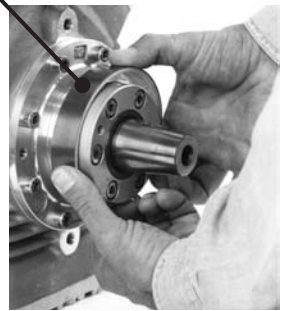
Leak oil collection ring
