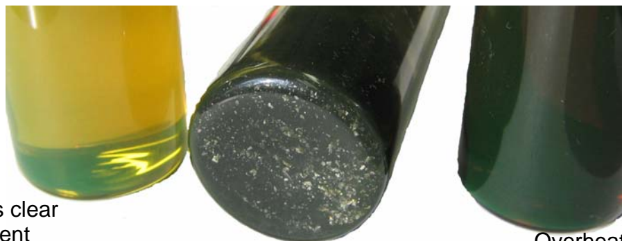
Example of contamination collected on inlet side of orifice tube requiring system flushing
