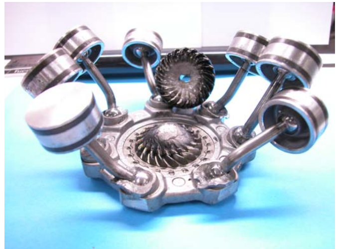
Overheated center ball and gear set
