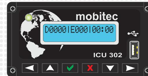
To access the control unit menu, press  $\checkmark$ . Move the button  $\triangleleft$  until the message below is displayed, press  $\checkmark$  to access the menu or cancel it by pressing  $\times$ .
