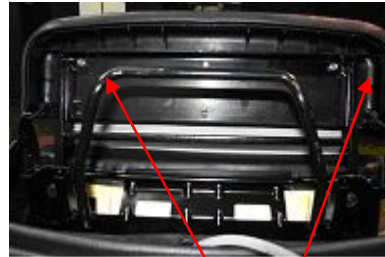
2. Ten-millimeter lock nuts on underside of thigh extension.
