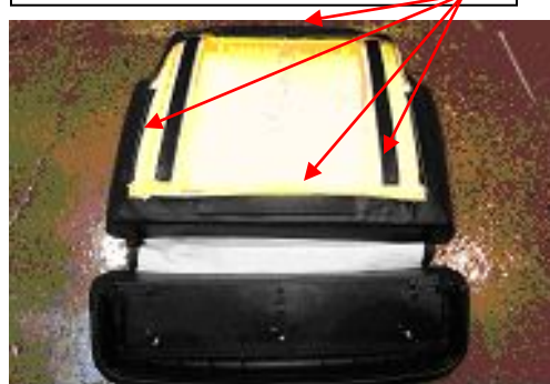
4. Seat cushion removed, undo Velcro sides to remove cushion.
