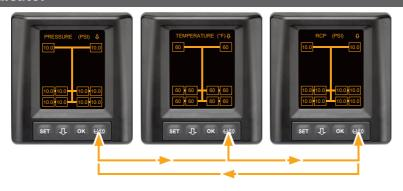
• Press the (1)/(1) button to switch between the pressure indicator, temperature indicator and the target pressure indicator.
