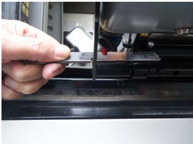
FIGURE 2-5: BRIDGEPLATE HEIGHT GAUGE TOOL SHOWN FOR CONFIG F9TF-DE019, F9TH-DE035
