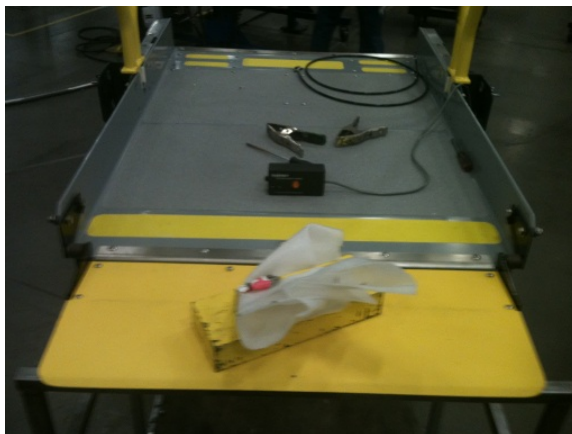
FIGURE 2-8. 25 LB. (11 KG) LOAD TEST (CENTER SIDE)
