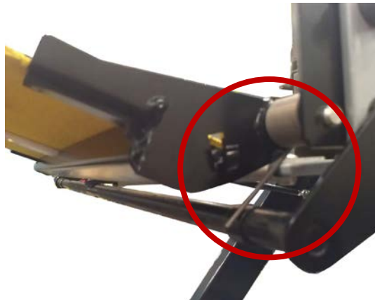
FIGURE 2-10. UNHOOK BRIDGEPLATE SPRING
