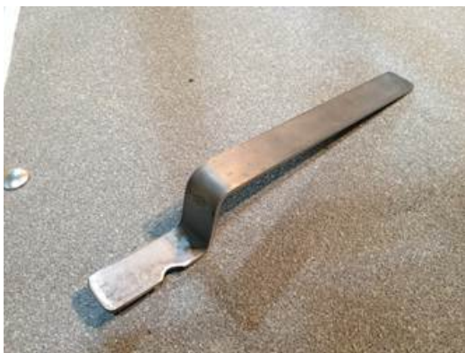
FIGURE 2-2A: HEIGHT GAUGE TOOL (P/N 56279)
