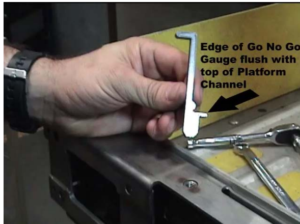
FIGURE 4-5: ROLLSTOP ADJUSTMENT TOOL P/N 55273
