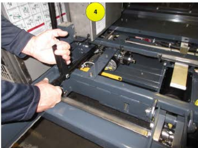
Release lift by engaging the manual release handle counter clockwise
