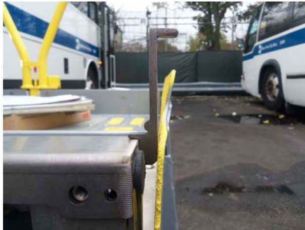
FIGURE 4-24: ROLLSTOP ADJUSTMENT TOOL P/N 55273
