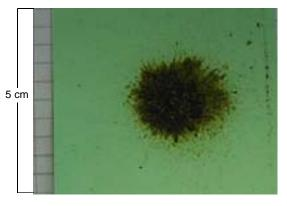
Dark spots on the paper alone do not indicate increased oil consumption of the compressor because carbon may have collected and settle on the paper. It is important whether the paper is dry or damp.
