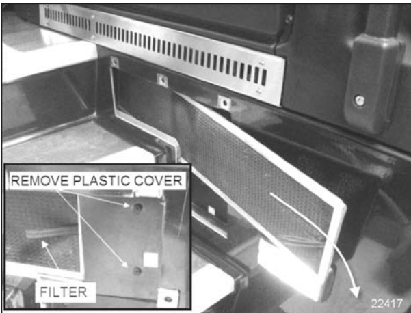
FIGURE 23: REMOVING DRIVER'S SECTION AIR FILTER
